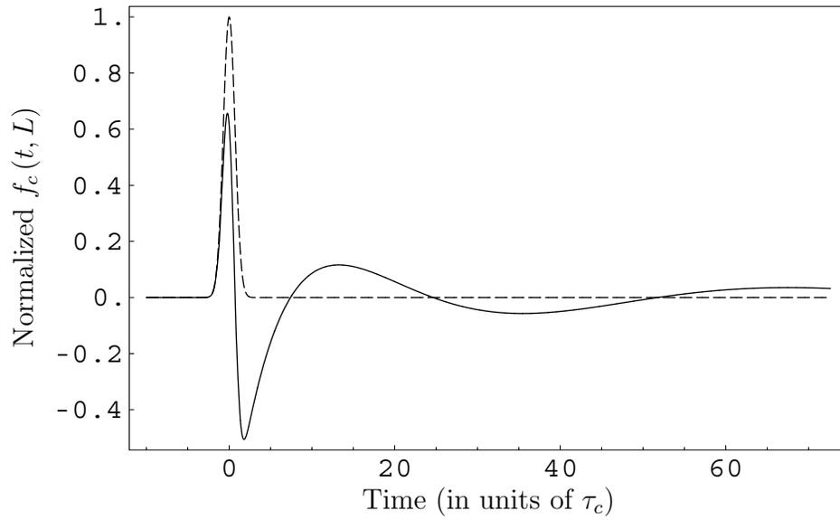
Figure 1.7: Normalized field envelope at  $y = 0$  (dashed) and at  $y = L$  (solid). For  $e_{disp} = 1$ , the ultrashort pulse experiences severe distortion, and develops an oscillatory structure to satisfy the vanishing pulse area theorem. The field is given by  $f_c(t, 0) = e^{-(t/\tau_c)^2}/\sqrt{\pi}$ . The parameters are  $\theta_c = 0.1$ ,  $\Delta_c = 0$ , and  $e_{disp} = 1$ . For  $\Delta_{dop} = 0.6GHz$  and  $\tau_c = 100fs$ , this corresponds to  $\alpha_{dop}L \simeq 16500$ .
