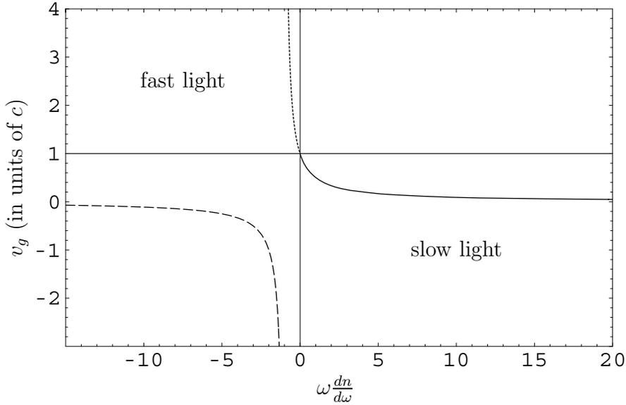
Figure 1.9: Slow, fast and backward propagating light. The origin is at  $(0, c)$ . The slow light regime is shown in solid, the fast light in dotted and dashed. The backward propagating is in dashed. For ultraslow light we need to have  $\omega dn/d\omega \gg 0$ .
