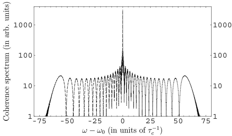
Figure 1.4: New frequency components generated during the action of light shifts with  $\omega_c = \omega_0$ . Each new component is generated twice, once when the levels are being stretched, and the second time when levels are relaxing back. The components at these two times interfere to give the modulated structure. The field is  $\Omega_c(t) = \Omega_{c0}e^{-(t/\tau_c)^2}$  with  $\Omega_{c0} = 60\tau_c^{-1}$ ,  $\Delta_c = 0$ .
