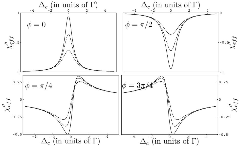
Figure 4.6: Imaginary parts of the effective susceptibility  $\chi''_{eff}$  (in units of  $2\alpha_0/k$ ) showing phase control of the medium response when  $|\Omega_c| \ll \sqrt{\Gamma_d\Gamma}$  is not satisfied. Parameters are  $\Omega_c = 0.1\Gamma$  (solid),  $0.3\Gamma$  (dashed), and  $0.5\Gamma$  (dotted). Other parameters are  $\Omega_p = 0.001\Gamma$ ,  $\Gamma_{ze} = 2\Gamma_d = \Gamma$ ,  $\Gamma_{zg} = 0$ , and  $\alpha_0 L = 0.2$ .
