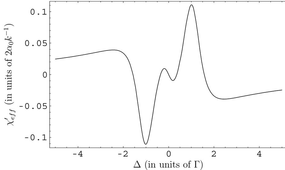
Figure 3.21: Anomalous dispersion at  $\Delta = 0$  suggests fast light propagation. Parameters are  $\Delta_c = 0$ ,  $\Omega_c = 0.6\Gamma$ ,  $\Gamma_d = 0.5\Gamma$ ,  $\Gamma_{zg} = 0$ , and  $\Gamma_{ze} = \Gamma$
