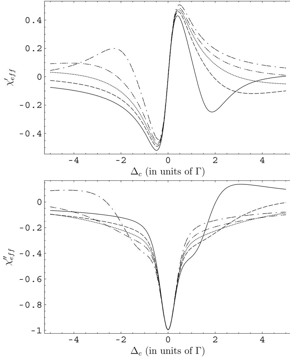
Figure 4.9: Susceptibility (in units of  $2\alpha_0/k$ ) behaves as  $\chi_{lin}^*$  close to resonance. Parameters are  $\phi = 0.5$  (solid),  $\phi = 1.0$  (dashed),  $\phi = 1.5$  (dotted),  $\phi = 2.0$  (dash dot dot), and  $\phi = 2.5$  (dash dot dash). Other Parameters are  $\Omega_c = 10^4\Omega_p = 0.1\Gamma$  (at entrance),  $\Gamma_{ze} = 2\Gamma_d = \Gamma$ , and  $\Gamma_{zg} = 0$ .
