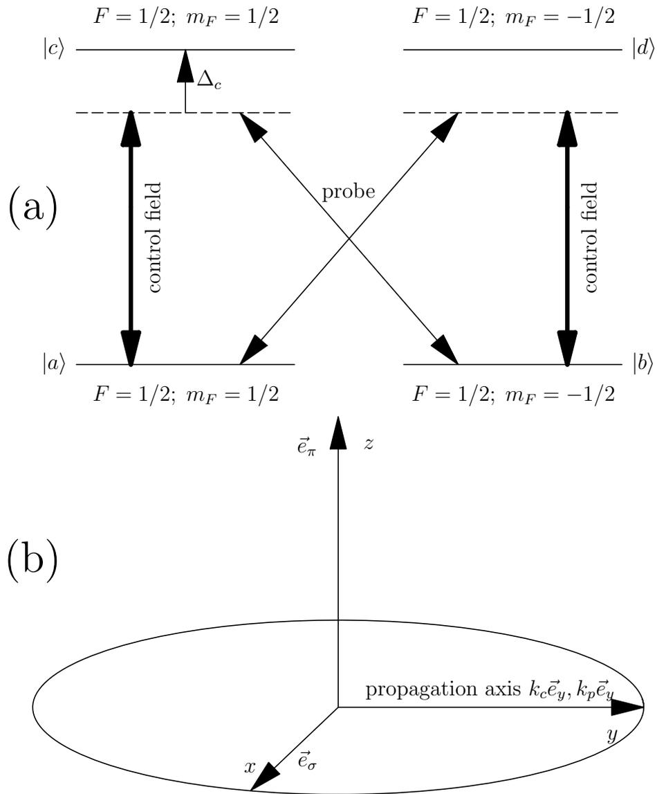
Figure 4.1: (a) A Double two-level system for the control of optical response of the medium. The  $\pi$  polarized control field drives each single two-level system, and the  $\sigma$  polarized probe connects crossed transitions. (b) Propagation and polarization axis.
