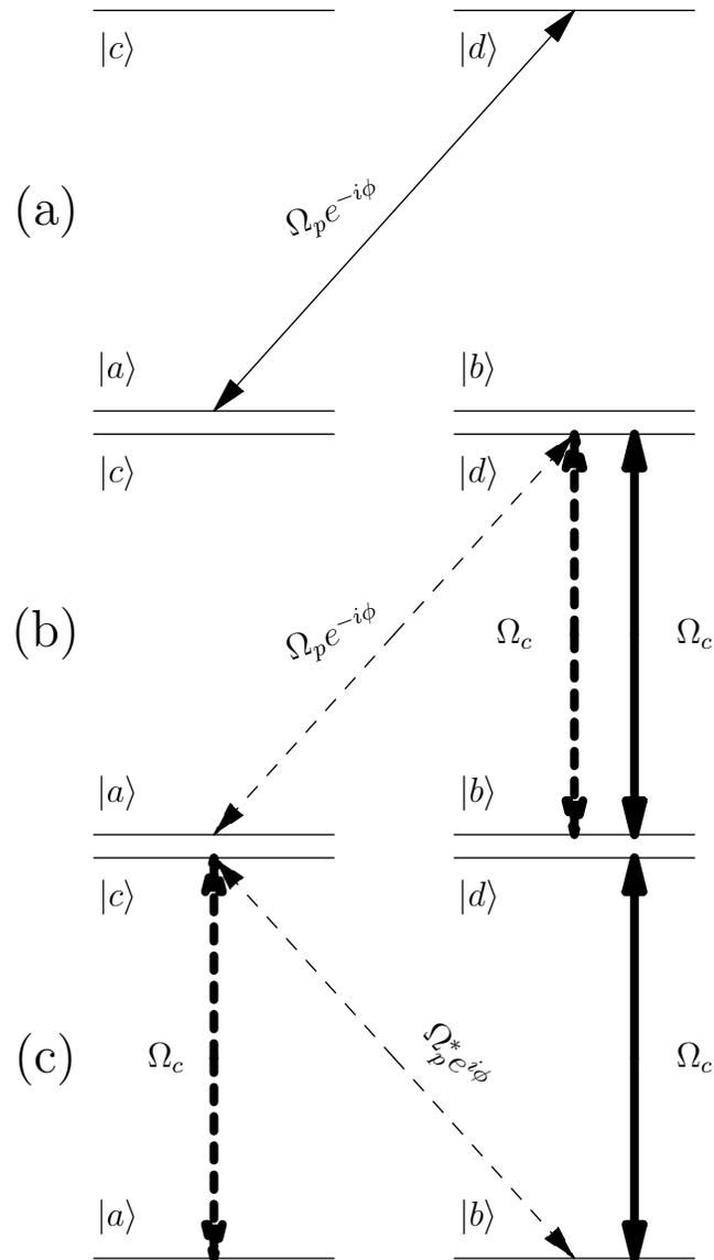
Figure 4.7: Quantum paths that give rise to  $\rho_{da}$ . (a) absorption by the population, (b) cross Kerr type path that compensates for the absorption, and (c) phase conjugate type path responsible for the phase dependence of the medium response.
