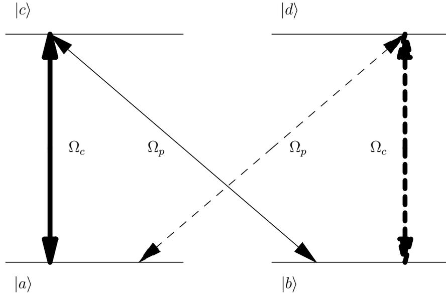
Figure 3.13: The double two-level system seen as a double  $\Lambda$  system. The control and the probe field in solid form one  $\Lambda$  system. The second system is shown with the control and the probe field in dashed.
