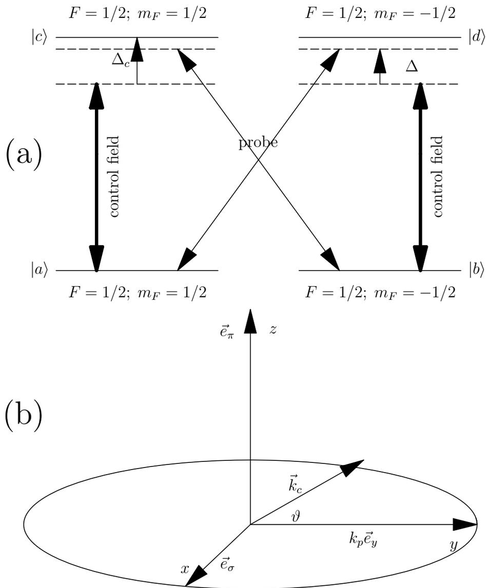
Figure 3.9: (a) A Double two-level system for slowing light. The  $\pi$  polarized control field drives each single two-level system, and the  $\sigma$  polarized probe connects crossed transitions. (b) Propagation and polarization axis.
