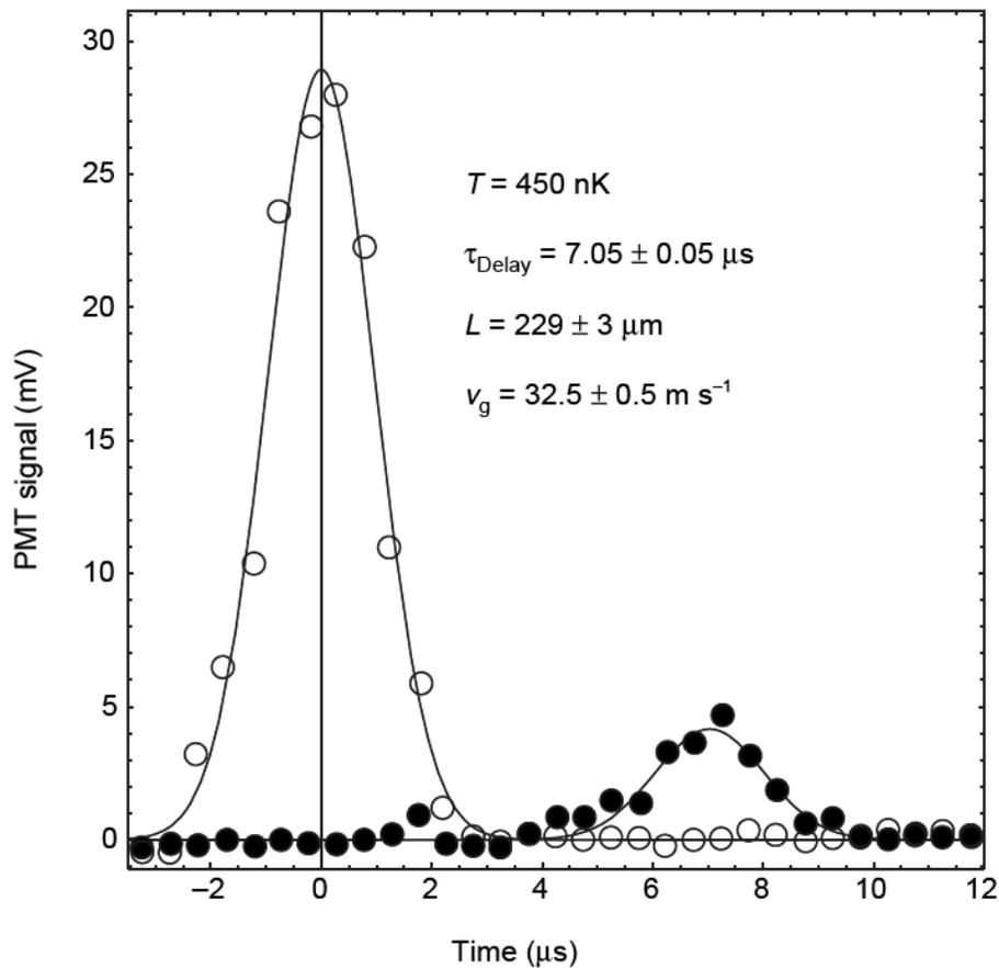
Figure 3.5: Slow light in ultracold sodium atoms(taken from [Hau99]). Open circles represent the reference probe when no atoms are present. Filled circles represent the probe delayed by  $7 \text{ } \mu\text{s}$  in a  $229 \text{ } \mu\text{m}$  medium, corresponding to  $v_g = 32.5 \text{ m/s}$ .
