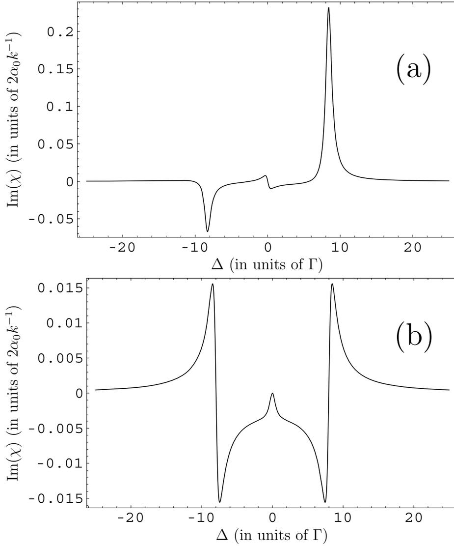
Figure 3.17: Absorption spectra when the system reduces to an effective (strongly driven) two-level system. Parameters are (a)  $\Delta_c = 2.5$ , (b)  $\Delta_c = 0$ . Other parameters are  $\Omega_c = 4\Gamma$ ,  $\Gamma_d = 0.5\Gamma$ ,  $\Gamma_{zg} = 0$ , and  $\Gamma_{ze} = \Gamma$
