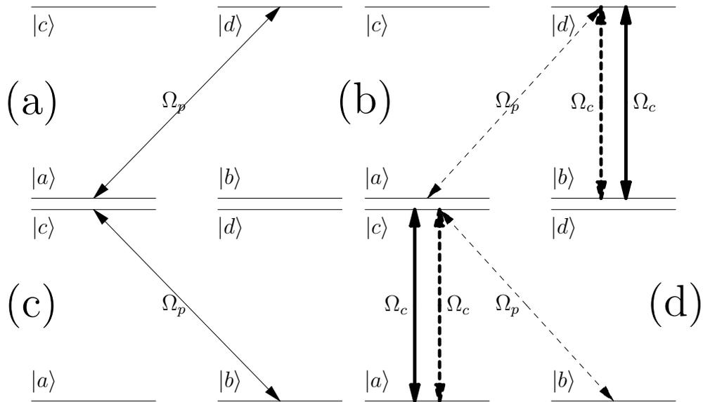
Figure 3.12: Quantum paths that contribute to generation of  $\rho_p^{(-)}$ . (a) Absorption path for  $\rho_{da}^{(-)}$ , (b) compensation path for  $\rho_{da}^{(-)}$ , (c) absorption path for  $\rho_{cb}^{(-)}$ , and (d) compensation path for  $\rho_{da}^{(-)}$ .
