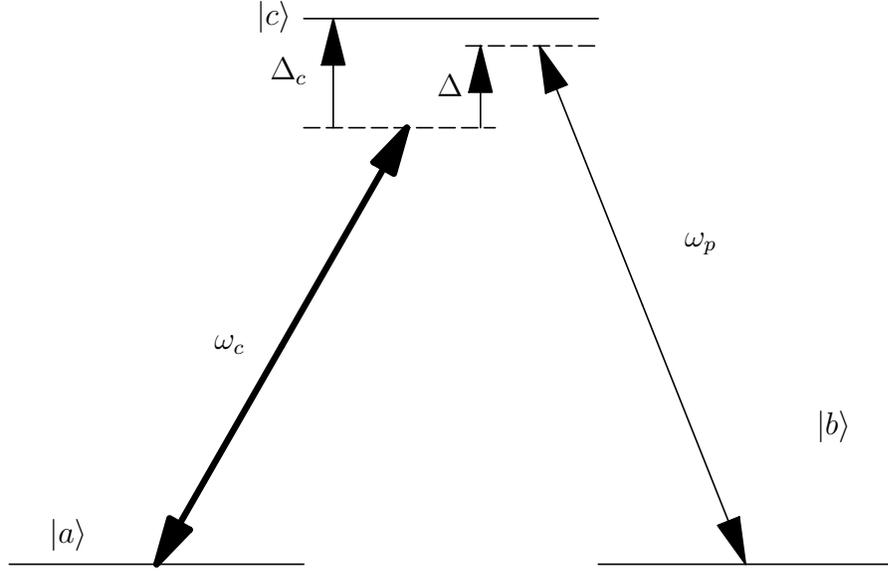
Figure 3.1: Three level  $\Lambda$  system for EIT.
