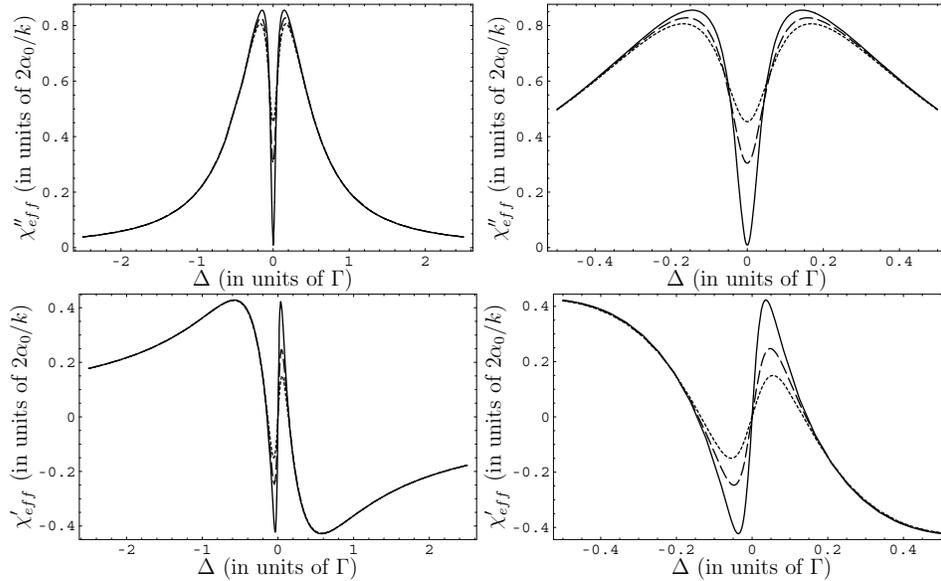
Figure 3.23: Decoherence between the ground Zeeman states spoils the transparency. Parameters for the four figures are (dotted)  $\Gamma_{zg} = 2\Omega_c^2/\Gamma_d$ , (dashed)  $\Gamma_{zg} = \Omega_c^2/\Gamma_d$ , and (solid)  $\Gamma_{zg} = 0.02\Omega_c^2/\Gamma_d$ . Other parameters are  $\Omega_c = 0.1\Gamma$ ,  $\Delta_c = 0$ , and  $2\Gamma_d = \Gamma_{ze} = \Gamma$ .
