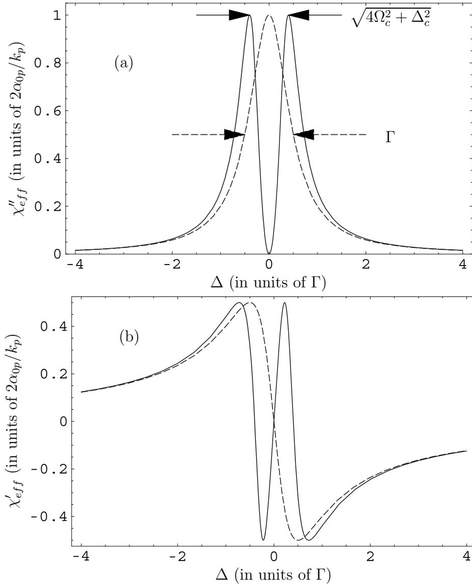
Figure 3.2: (a) Absorptive and (b) dispersive response of the medium for the probe in the presence  $\Omega_c = 0.4\Gamma$  (solid), and absence  $\Omega_c = 0$  (dashed) of the control. Other parameters are:  $\Delta_c = 0$  and  $\Gamma_d = 0.5\Gamma$ .
