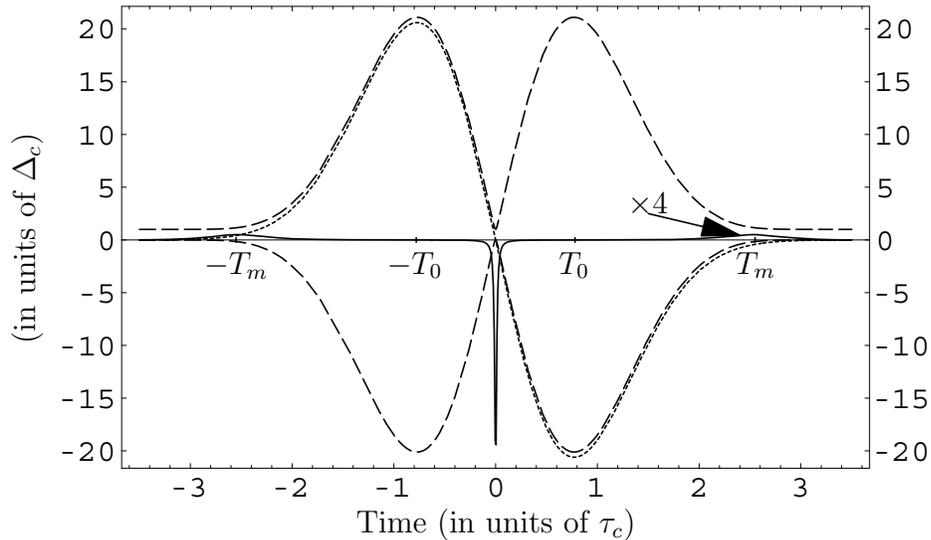
Figure 2.7: Field profile (dotted), adiabatic energy levels (dashed), and (4 times) magnified non-adiabatic coupling (solid). The coupling presents a minimum at  $t = 0$ , is 0 at  $t = \pm T_0$ , and presents two local maxima at  $t = \pm T_m$ .
