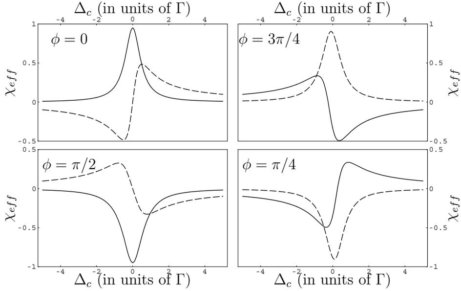
Figure 4.5: Real (dashed), and imaginary (solid) parts of the effective susceptibility (in units of  $2\alpha_0/k$ ), showing phase control of the medium response. Parameters are  $\Omega_c = 100\Omega_p = 0.1\Gamma$ ,  $\Gamma_{ze} = 2\Gamma_d = \Gamma$ ,  $\Gamma_{zg} = 0$ , and  $\alpha_0 L = 0.2$ .
