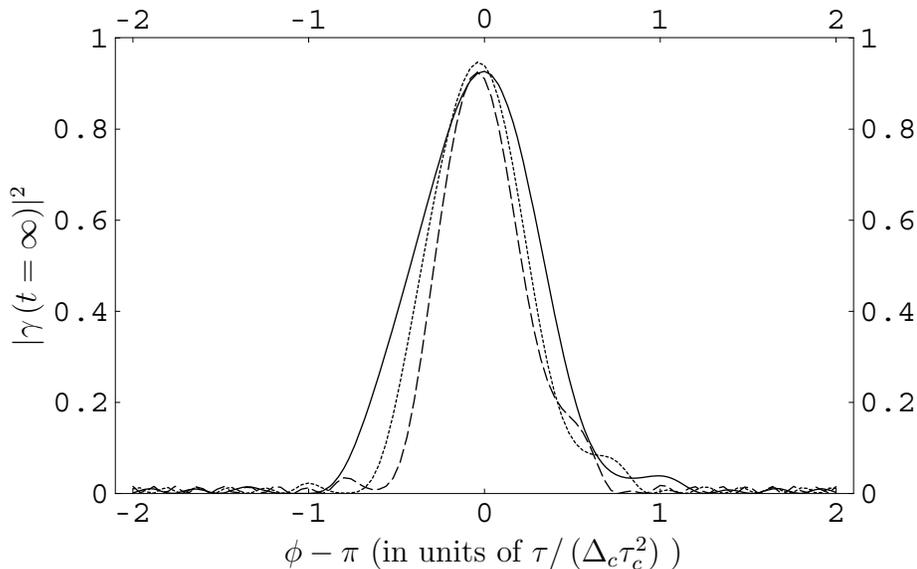
Figure 2.13: Sensitive phase dependence of NRJ. FWHM of the central peak decreases with increasing  $r$ . Parameters are  $r = 50$  (solid) with width  $0.031\pi$ ,  $r = 75$  (dotted) with width  $0.025\pi$ , and  $r = 100$  (dashed) with FWHM given by  $0.019\pi$
