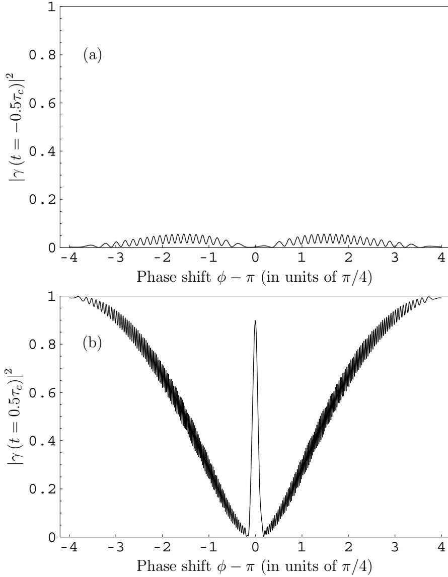
Figure 2.9: Adiabatic excited state population profile (a) before NAJ at  $t = -0.5\tau_c$ ; (b) after NAJ at time  $t = 0.5\tau_c$ . NAJ exists only for  $\phi$  very close to  $\pi$ . Away from  $\phi = \pi$ , population in (a) is due to non-resonant coupling provided by  $V(\phi, t)$ ; and in (b) because of level crossings. The oscillations are discussed in the text. Parameters are  $\Delta_c = 8\tau_c^{-1}$ ,  $\vartheta_c = 400\tau_c^{-1}$  ( $r = 50$ ), and  $\tau = \tau_c$ .
