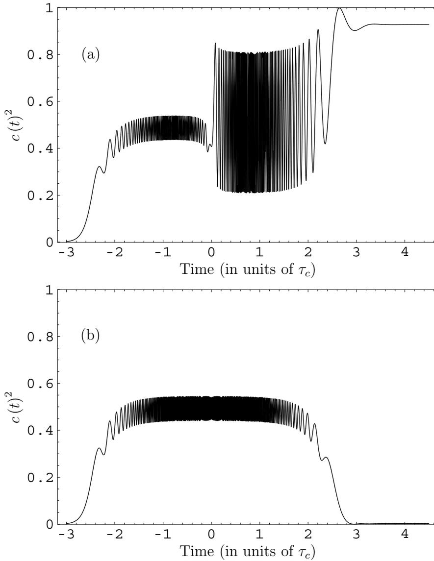
Figure 2.14: Excited bare state population corresponding to (a) NAJ in Fig. 2.8 with  $\phi = \pi$ , and (b) ARP in Fig. 2.12(b) with  $\phi = 0$ . In (a) the oscillation amplitude is changed with NAJ. In (b) the complete population inversion in adiabatic basis gets unnoticed in bare state representation. Parameters are  $\Delta_c = 8\tau_c^{-1}$ ,  $\vartheta_c = 400\tau_c^{-1}$  ( $r = 50$ ),  $\tau = \tau_c$ , and  $\phi = \pi$ .
