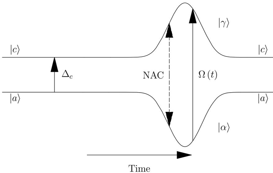
Figure 1.2: Two level system in adiabatic bases. The bare states are separated by  $\Delta_c$  (after RWA). The strong field stretches the levels apart for transient time. The separation between the levels is proportional to  $\Omega(t)$ , and the transitions between the levels are provided by non-adiabatic coupling (NAC)
