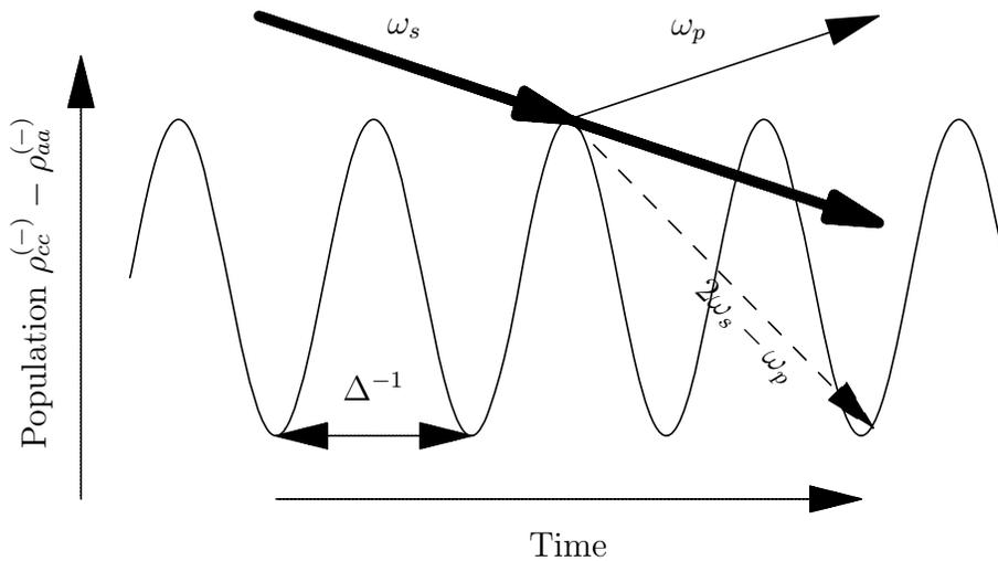
Figure 3.8: Compensation for the absorption of probe. Diffraction of the control field from the population grating compensates for the absorption of probe. A small angle between the control and the probe is required (for  $\Delta = 0$ ) to separate spatially the component that radiates at  $2\omega_s - \omega_p$  frequency.
