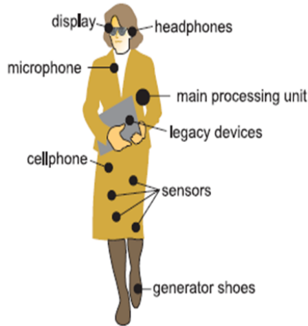
Figure 3.3 – The body area computing system for wearable computers
