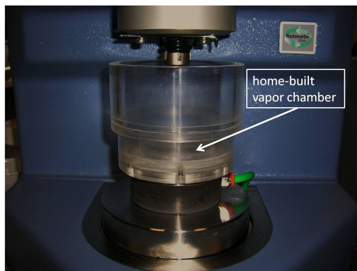
Fig.3.3: Water chamber to prevent evaporation.
