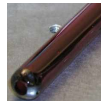
Fig. 2. (b) chalcogenide tube formed by rotational casting
