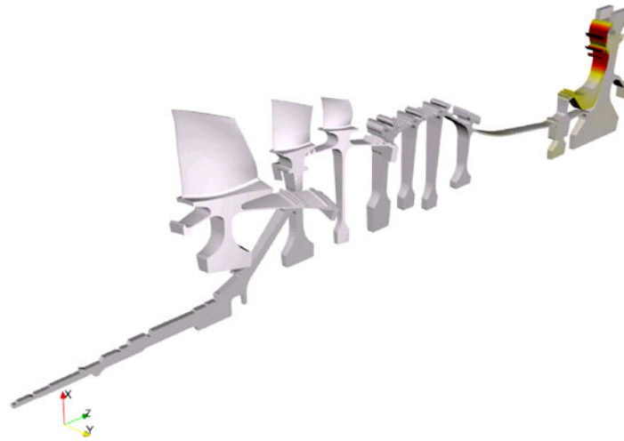
Figure 2.46: Mono-harmonic eigensolution localized to the seal with \delta = 1 at f = 16.33 [FSHP]
