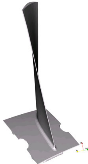
Figure 3.11: Geometry of the booster blade
