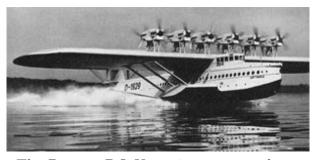
The Dornier DO-X, a 12 engine seaplane, able to transport 169 passengers, 1929
