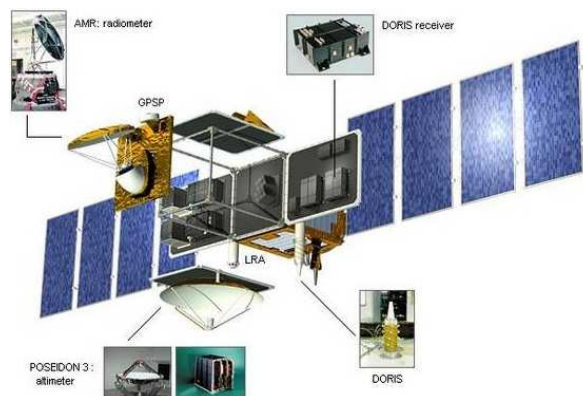
Figure 2.2.: Exploded view of the Jason 2 satellite and its main payloads. The T2L2 optics are mounted on the boom that holds the LRA (image center); the T2L2 electronics are mounted on the X+ wall of the satellite, next to the DORIS system.
