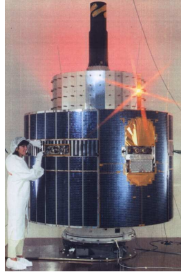
Figure 2.1.: The Meteosat-P2 satellite with the LASSO payload (front of main cylinder): The lower part is the retroreflector panel, the upper the detection system (photograph taken from [12]).
