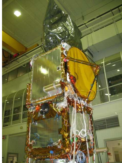
Figure 3.25.: Jason 2 during integration in the THALES Alenia Space satellite integration clean hall: The LRA pyramid may be discerned in the center, left to the big Poseidon antenna. The T2L2J2 optics are situated just left of the LRA.
