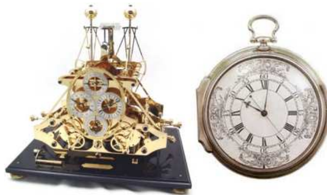
Figure 1.1.: The first Harrison chronometer H1 (1735) and his masterpiece H4 (1759). Captain James Cook took an exact copy of the H4, Kendall’s K1, on his second journey into the south Pacific and ascertained its excellent quality to the British admiralty, what finally led to the recognition of the “Longitude Prize” to Harrison. Photographs © National Maritime Museum, UK
