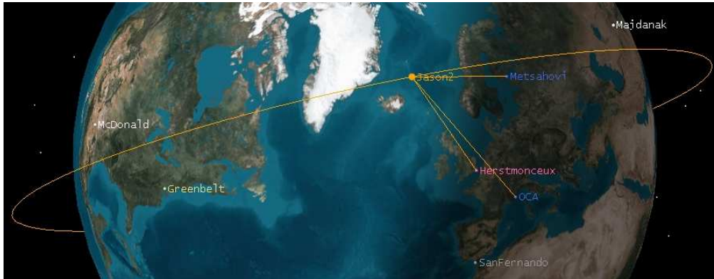
Figure 5.18.: A transatlantic time transfer may be assisted by the English Herstmonceux or the Finnish Metsahovi station
