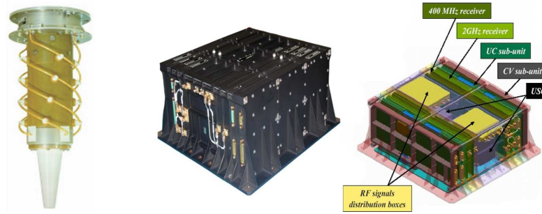
Figure 2.6.: The DORIS satellite payload on Jason 2: On the left, the combined 2 GHz and 400 MHz antenna, on the right the DGxx (USO and receiver). Photographs and CAD-view © CNES, France
