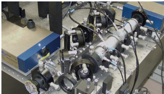
Figure 3.2.: The HighQ laser and the set of two pulse pickers as configured in the test setup
