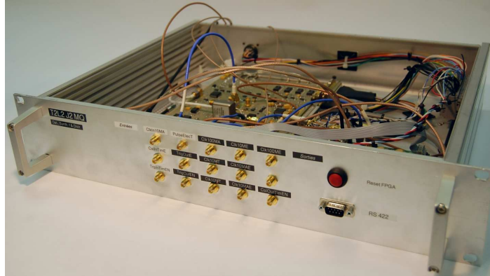
Figure 3.18.: A versatile frequency synthesis and signal distribution device based on T2L2 prototype boards
