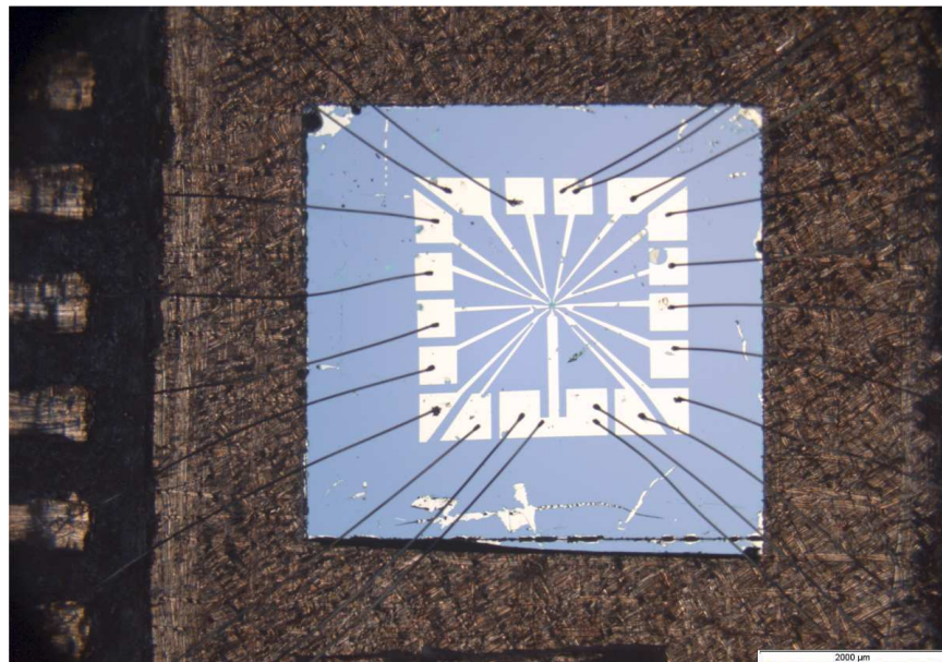
Figure 4.4: Typical fabricated sample glued to the sample holder and with bonded contacts.
