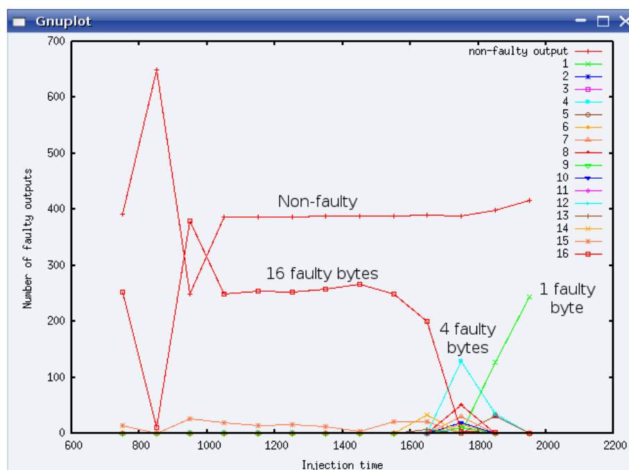
FIG. 4.7 – Faulty output bytes on AES
