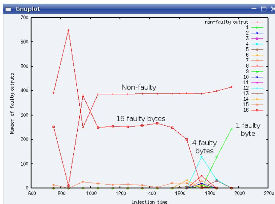
FIG. 4.7 – Faulty output bytes on AES
