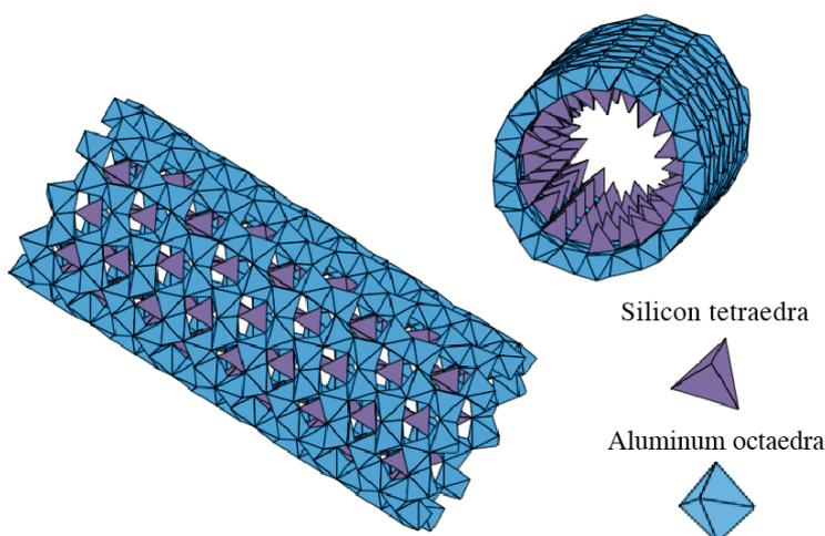
Figure 2. Imogolite structure.
