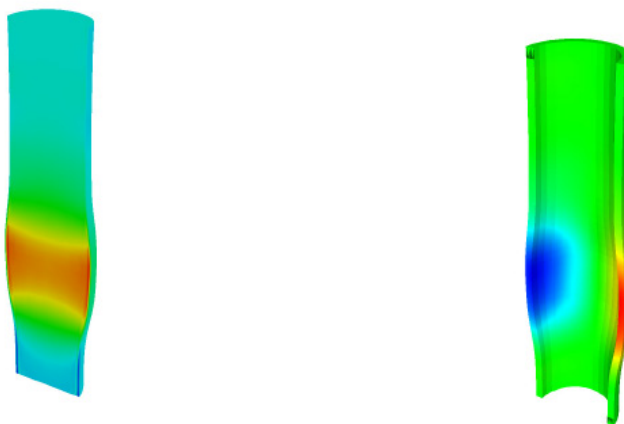
Fig. 3.10 Solution of the 3D model at t = 50.10^{-4} (left : fluid velocity, right : wall displacement)
