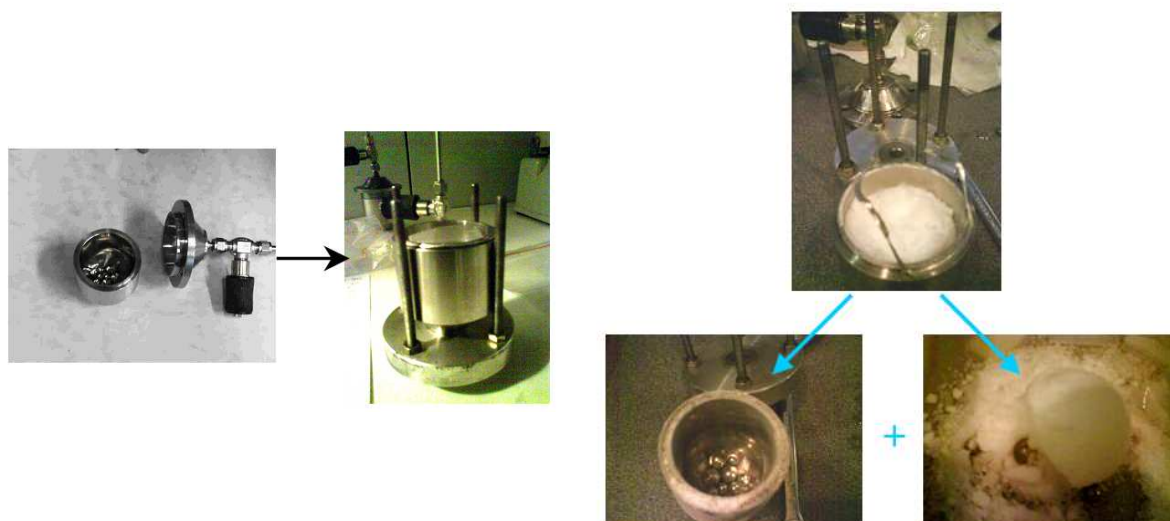
Fig. 3-1: ( left panel ): photos of ice mill before and after entering the sample with the dry extraction milling method; ( right panel ): photos of ice mill after milling
