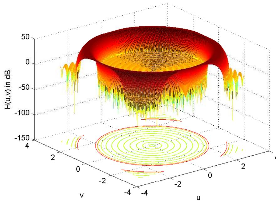
Figure 4.6: Magnitude response in dB of 20<sup>th</sup> order Chebyshev high pass FIR filter.
