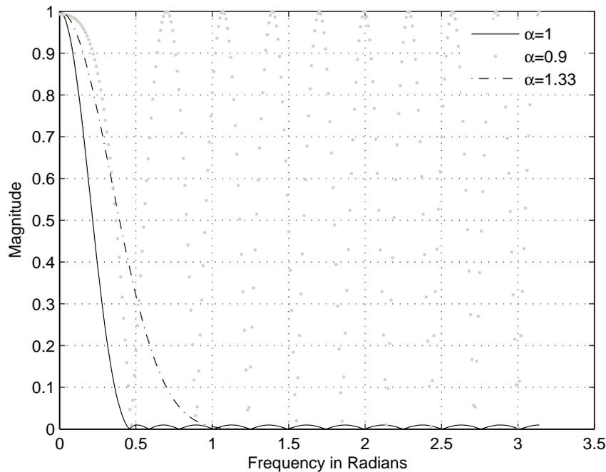
Figure 3.6: Magnitude response of 24<sup>th</sup> order Chebyshev low pass FIR filter.
