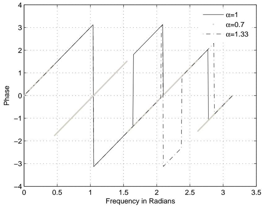
Figure 3.3: Phase response of 6<sup>th</sup> order Chebyshev low pass FIR filter.
