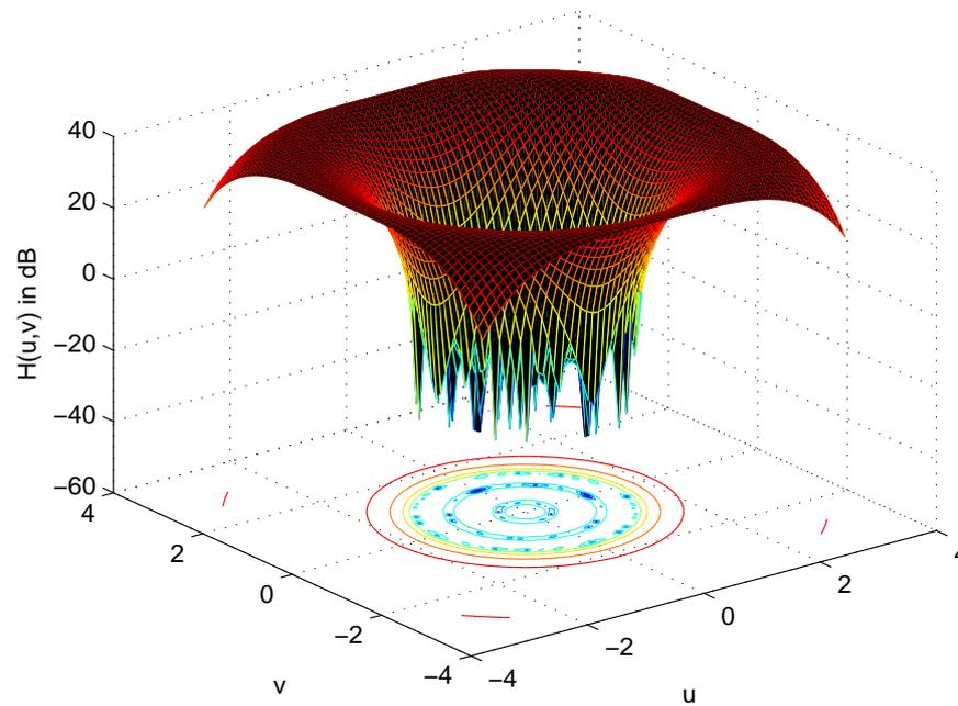
Figure 4.4: Magnitude response in dB of 6<sup>th</sup> order Chebyshev high pass FIR filter.
