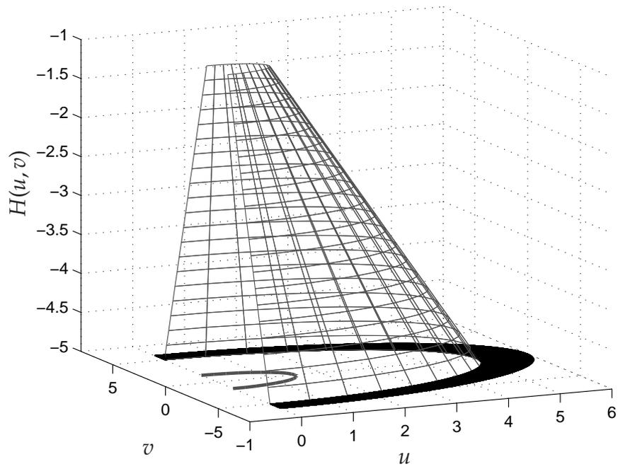
Figure 8.1: 3D desired low pass filter response.
