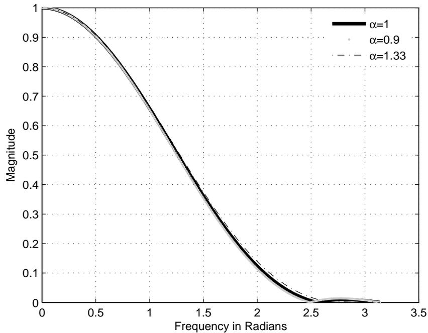
Figure 3.4: Magnitude response of 3<sup>rd</sup> order Chebyshev low pass FIR filter.
