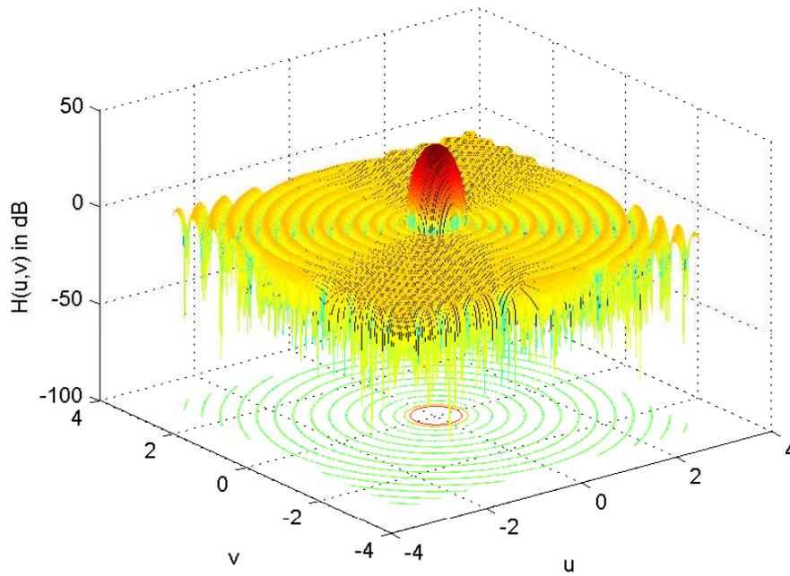
Figure 4.5: Magnitude response in dB of 20<sup>th</sup> order Chebyshev low pass FIR filter.
