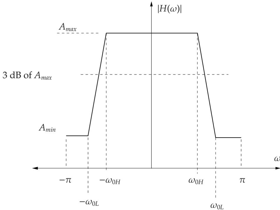
Figure 5.2: Desired characteristics of low pass filter.
