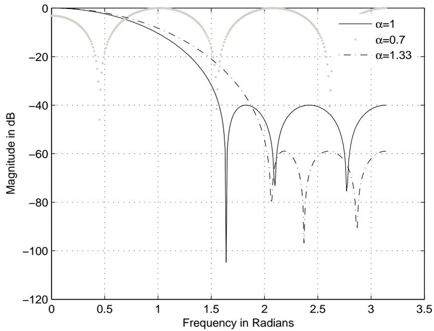
Figure 3.2: Magnitude response in dB of 6<sup>th</sup> order Chebyshev low pass FIR filter.
