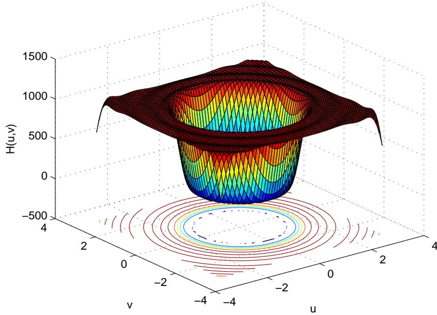
Figure 6.12: Magnitude response of high pass FIR filter when object function is approximated using 15 orthogonal polynomial terms.
