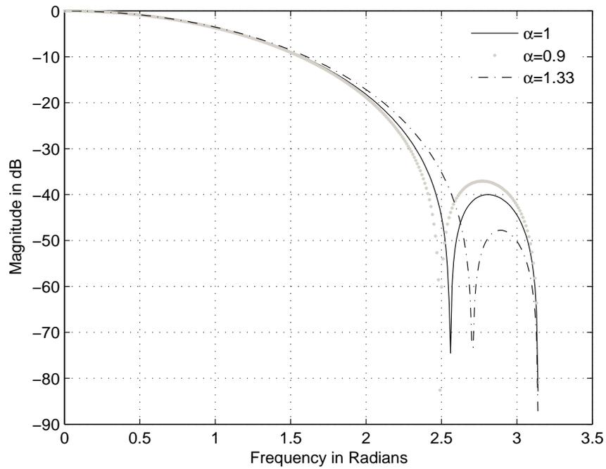
Figure 3.5: Magnitude response in dB of 3<sup>rd</sup> order Chebyshev low pass FIR filter.
