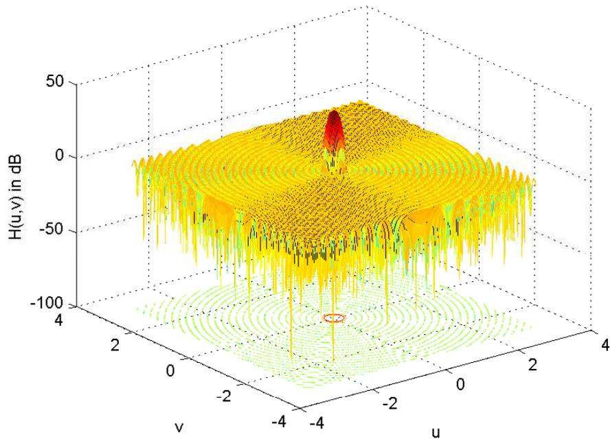
Figure 4.7: Magnitude response in dB of 40<sup>th</sup> order Chebyshev low pass FIR filter.
