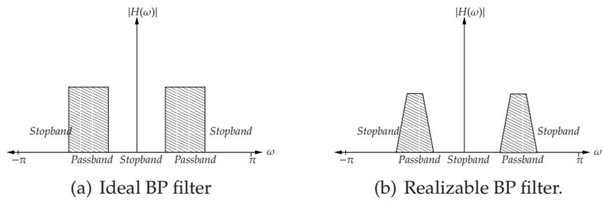
Figure 1.4: Band Pass (BP) filter.
