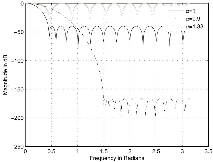
Figure 3.7: Magnitude response in dB of 24<sup>th</sup> order Chebyshev low pass FIR filter.
