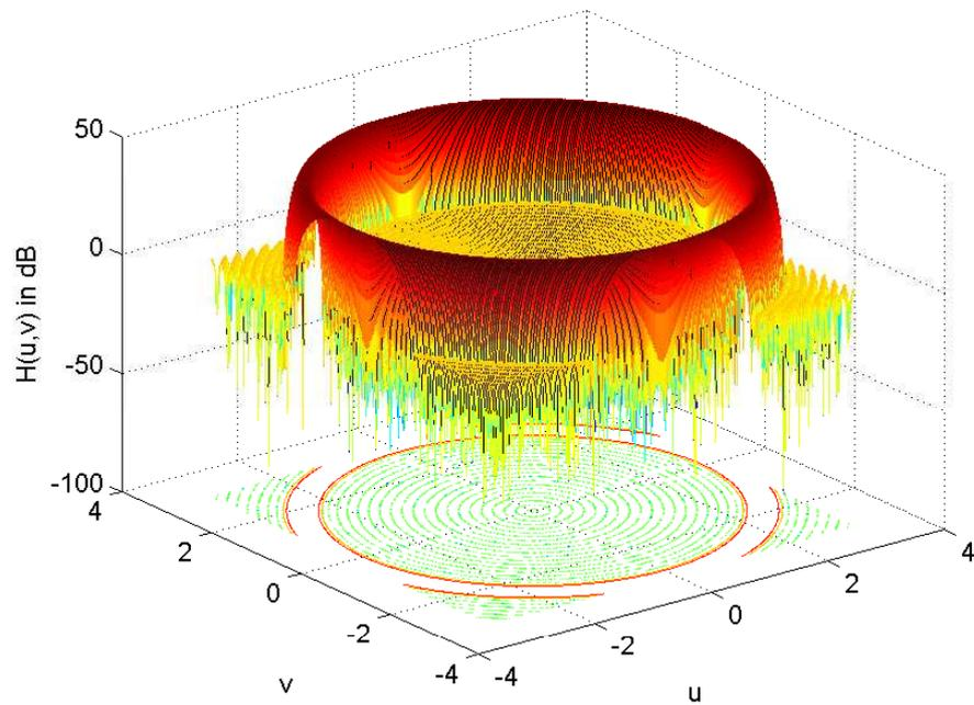
Figure 4.8: Magnitude response in dB of 40<sup>th</sup> order Chebyshev high pass FIR filter.
