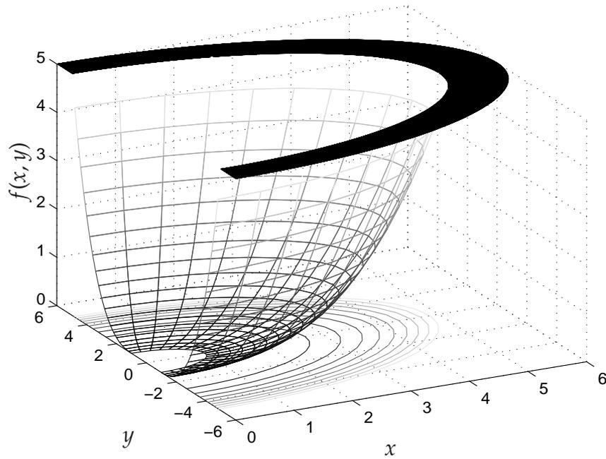
Figure 8.3: 3D object function for low pass filter of Figure 8.1, showing the slight non linearity in the transition region.
