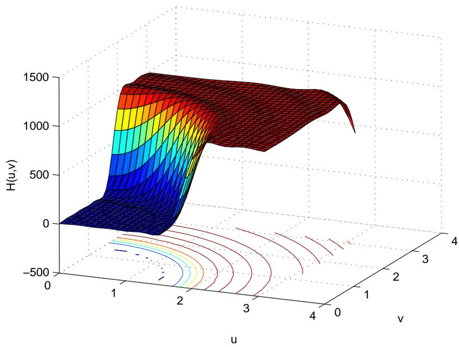
Figure 6.13: Cross section of magnitude response of high pass FIR filter when object function is approximated using 15 orthogonal polynomial terms.
