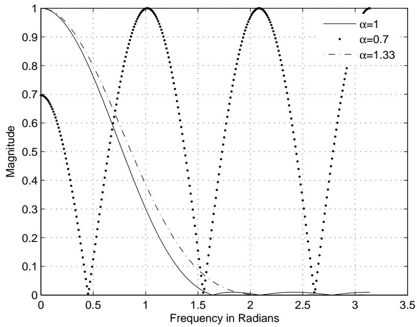
Figure 3.1: Magnitude response of 6<sup>th</sup> order Chebyshev low pass FIR filter.
