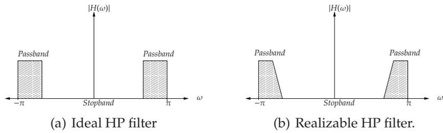
Figure 1.3: High Pass (HP) filter.
