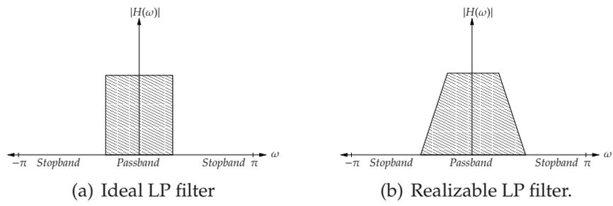
Figure 1.2: Low Pass (LP) filter.
