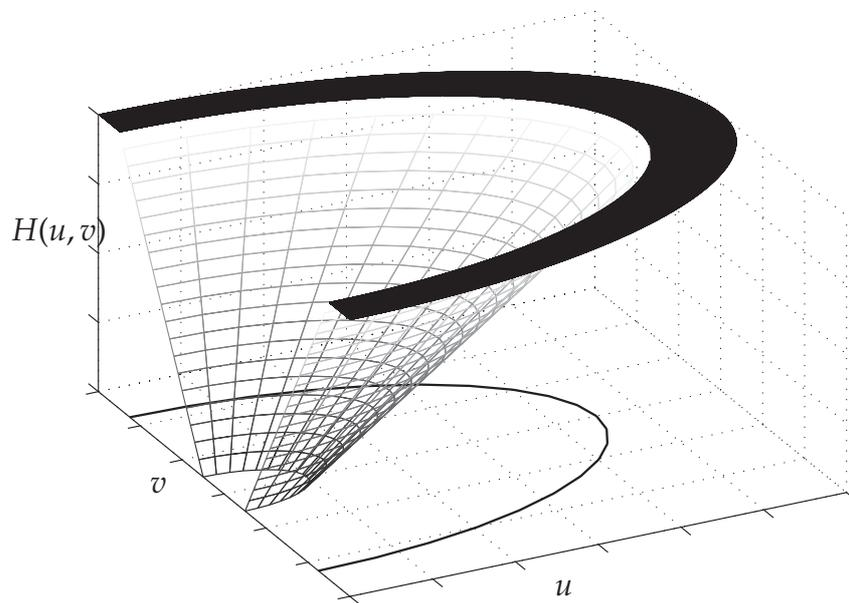
Figure 8.2: 3D desired high pass filter response.
