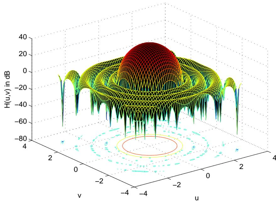
Figure 4.2: Magnitude response in dB of 6<sup>th</sup> order low pass FIR filter.
