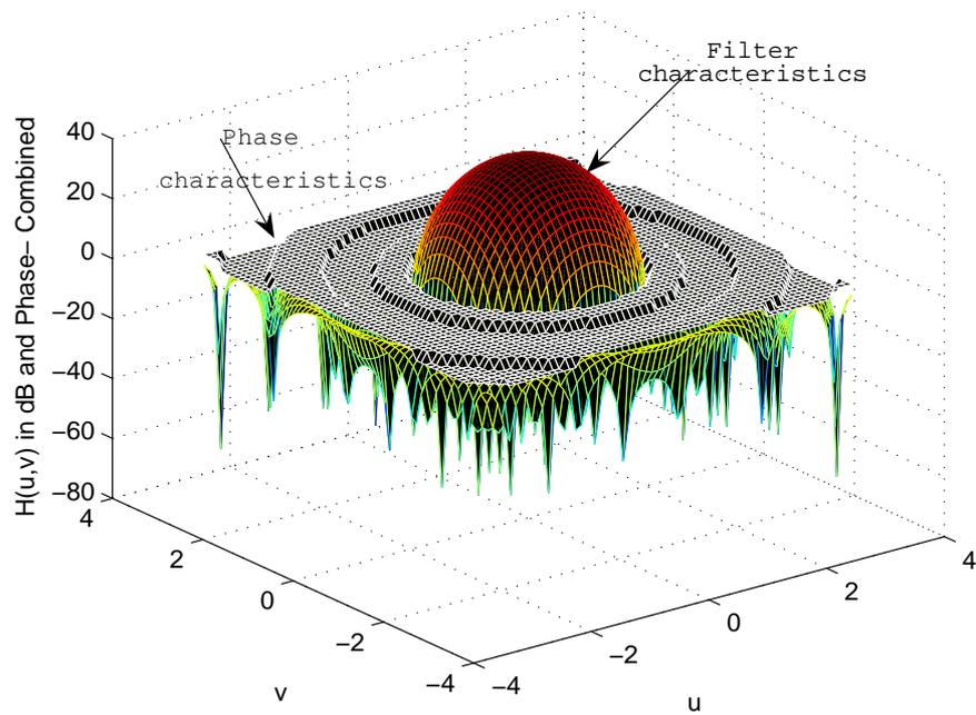
Figure 4.3: Phase response of 6<sup>th</sup> order low pass FIR filter.
