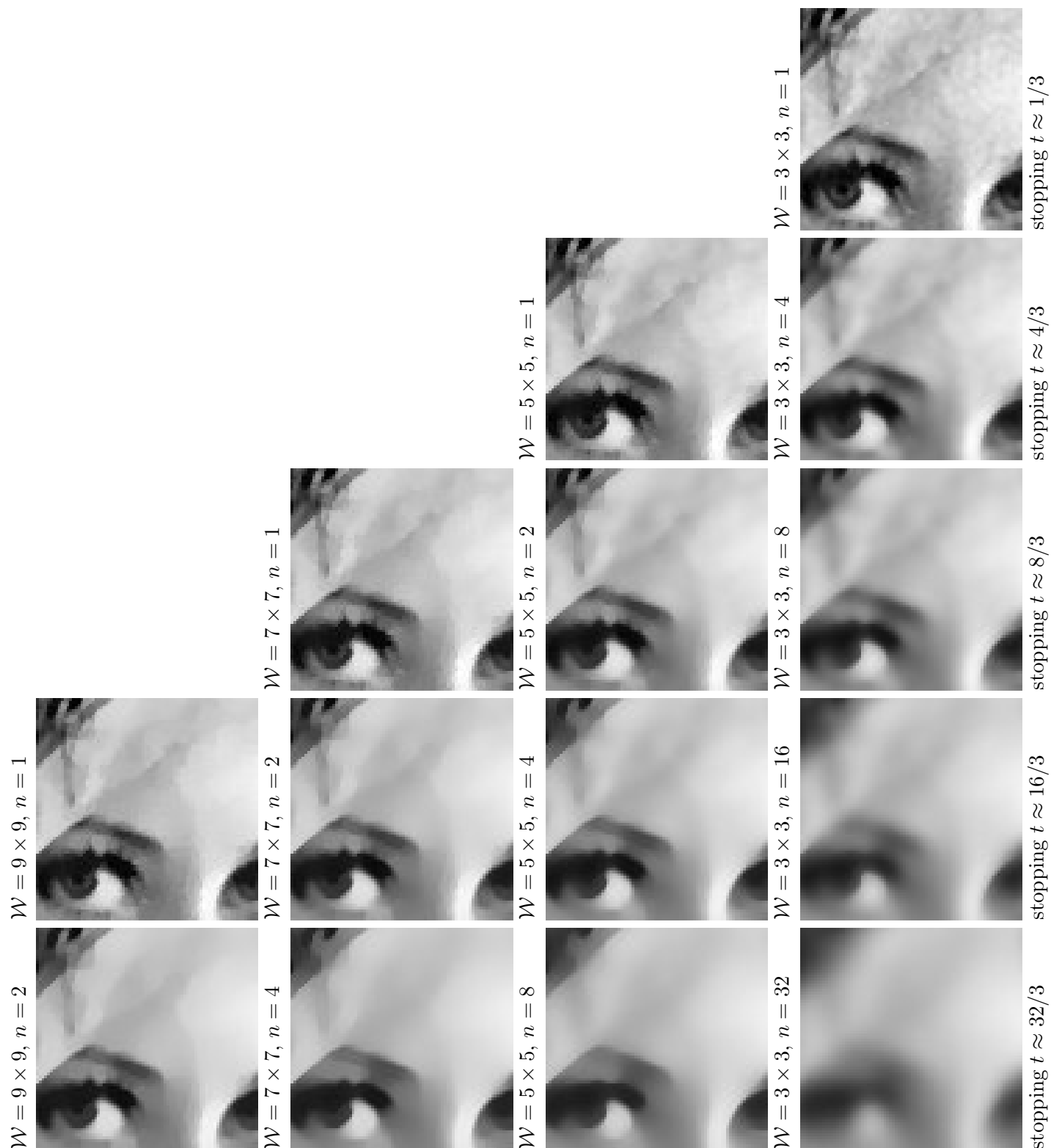
Figure 5.4: Iterated local TV-MAP. The window with radius h and the number n of iterations are such that nh^2/6 is approximately constant on each row. Going to the right means increasing values of n and decreasing values of h .
