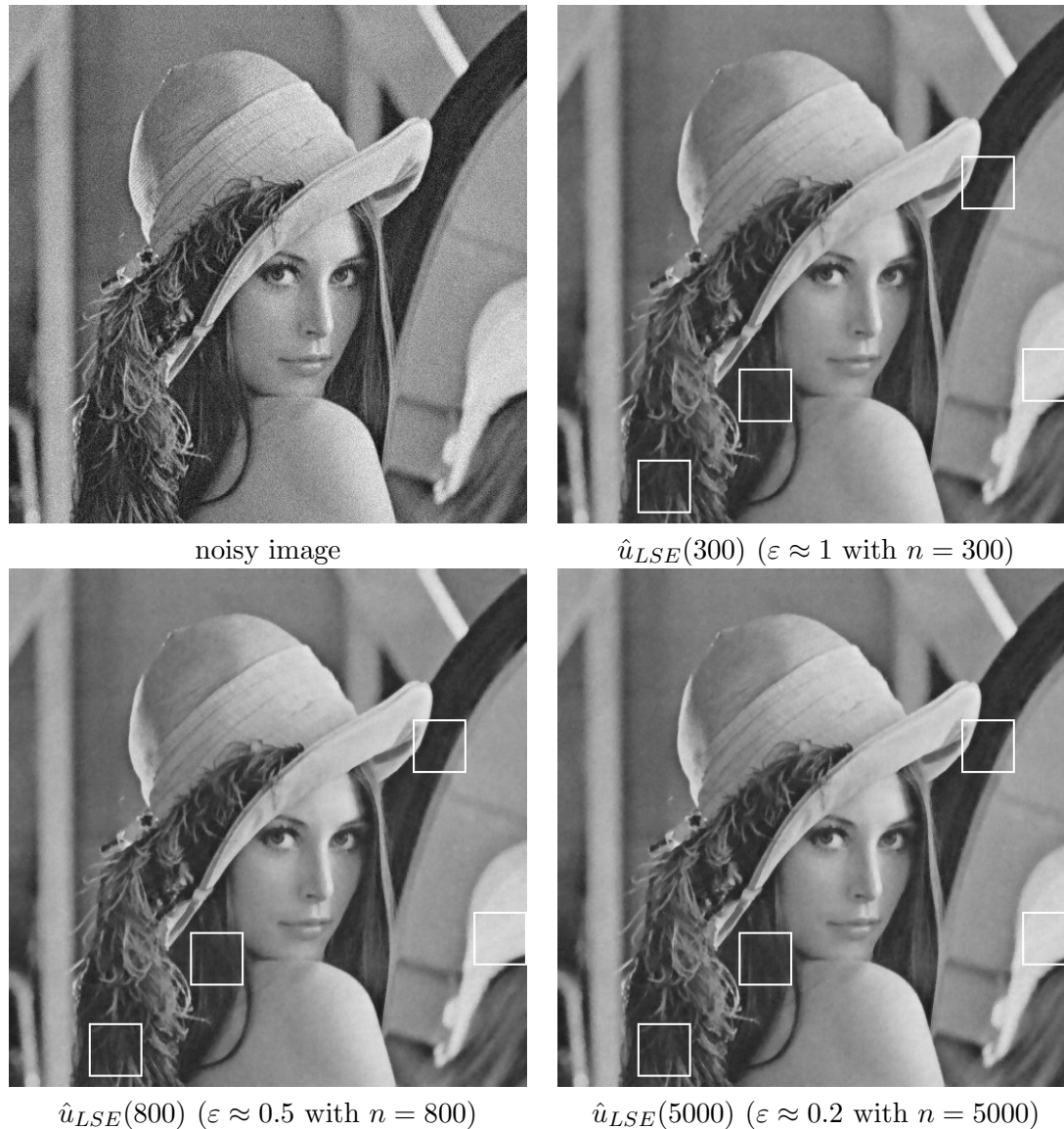
Figure 4.1: Influence of \varepsilon in the stopping criterion (I). The Lena image (with gray levels inside [0, 255] ) noised by a Gaussian white noise with standard deviation (s.d.) \sigma = 10 (top-left image) is denoised using TV-LSE with the algorithm explained in Chapter 2. The three other images are the partial averages (S_n^b + \tilde{S}_n^b)/2 of a unique run of the algorithm, for three values of n . The parameters are all fixed ( \sigma = 10 , W = 30 , \alpha = 27 , no burn-in) except from the number of iterations n . The top-right image, named \hat{u}_{LSE}(300) , obtained by a 300-iteration run, is such that the distance between the 2 chains of the algorithm \|S_{300}^0 - \tilde{S}_{300}^0\| is closest to 2, so that we expect the image to be at a distance \varepsilon \approx \|S_{300}^0 - \tilde{S}_{300}^0\|/2 \approx 1 from the true TV-LSE denoised image \hat{u}_{LSE} (actually n = 300 corresponds to the multiple of 50 reaching the distance closest to 2, because the images of the MCMCs were saved only every 50 images). Waiting for some more iterations yields the bottom-left image \hat{u}_{LSE}(800) ( \varepsilon \approx 0.5 with n = 800 ), and the bottom-right image \hat{u}_{LSE}(5000) ( \varepsilon \approx 0.2 with n = 5000 ). The three images look the same, it is difficult to make them apart, even on the zooms presented on next figure. For this 512 \times 512 image, one must count 166 seconds, i.e. almost 3 minutes to run 100 iterations of the algorithm (for the two 512^2 -subsampled chains).
