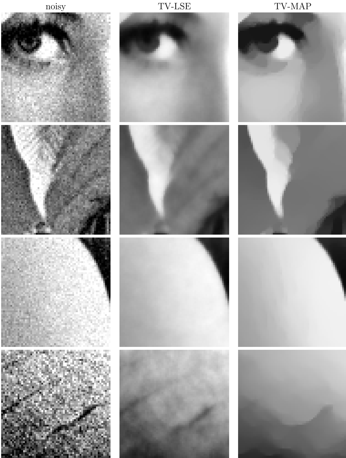
Figure 4.20: (I) High level of denoising ( \|\hat{u} - v\| = 13.06 for the Lena image noised by a Gaussian noise with s.d. = 10). An affine contrast change (unique for each line) has been applied on all the images of Figures 4.20 to 4.22 in order to improve the visibility of details. First column: details of the noisy image. Second column: TV-LSE denoising with parameters (\lambda, \sigma) = (100, 20) . The noise has been removed. A very slight blur has erased some fine textures, but the global aspect is nice. Third column: TV-MAP denoising with parameter \lambda_{MAP} = 73.1 . The noise has been removed while the edges remain well localized. However the ubiquitous staircasing effect over-simplifies the images and maintain an artificial aspect to these (the bottom image for instance is definitely damaged).
