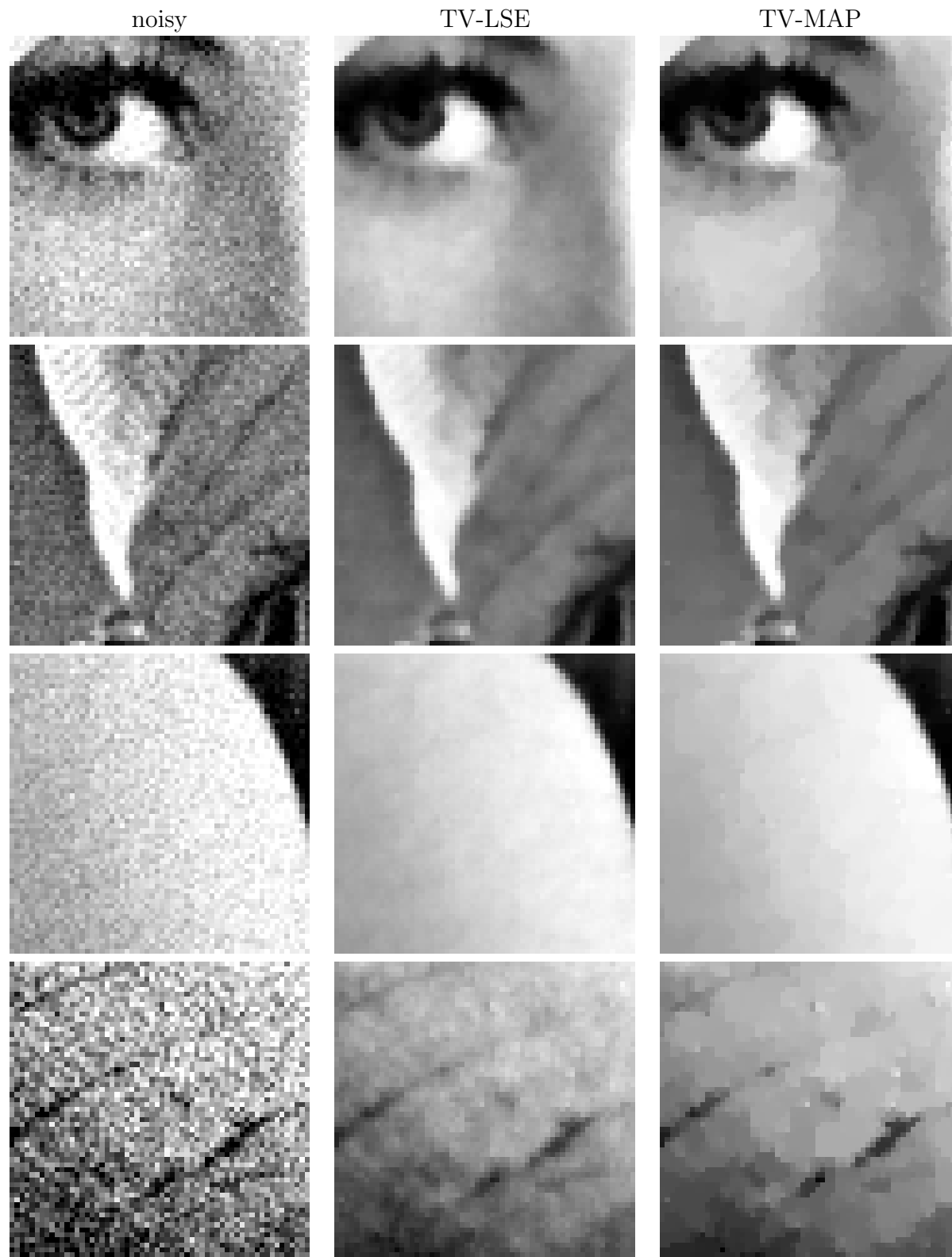
Figure 4.17: (I) Middle level of denoising ( \|\hat{u} - v\| = 9.33 for the Lena image noised by a Gaussian noise with s.d. = 10). An affine contrast change (unique for each line) has been applied on all the images of Figures 4.17 to 4.19 in order to improve the visibility of details. This is why some gray levels are saturated. First column: details of the noisy image. Second column: TV-LSE denoising with parameters (\lambda, \sigma) = (30, 10) . Texture is quite well recovered, as well as edges and homogeneous regions which really look natural. Some noisy texture remains. Third column: TV-MAP denoising with parameter \lambda_{MAP} = 17.3 . A few contrasted isolated pixels are still visible, whereas staircasing becomes significant.
