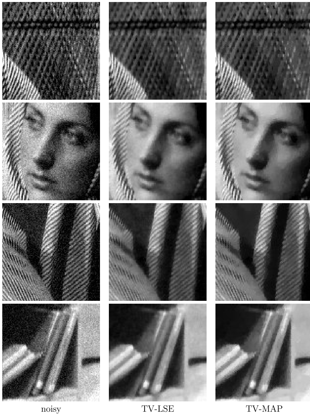
Figure 4.33: Examples on Barbara. On the first column, details of the degraded Barbara image are shown (Gaussian white noise with s.d. 10). The corresponding TV-LSE denoised images are shown on the second column ( (\lambda, \sigma) = (20, 10) ), and the TV-MAP denoised images on the third column ( \lambda_{MAP} = corresponding to the level of denoising of the LSE images).
