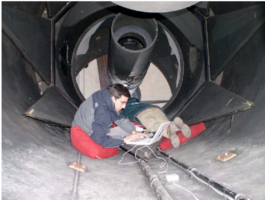
Figure 8.6: Working inside the UH88 tube. The baffling of SNIFS was made by covering different internal components using a black felt-like paper, and tested by making consecutive exposures using the photometric channel, controlling SNIFS directly from inside the tube.
