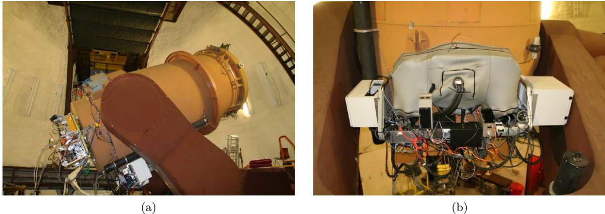
Figure 4.1: (a) University of Hawaii 2.2m (UH88) telescope; (b) SNIFS mounted on the bent-Cassegrain port of UH88. The main instrument is in the center under the neoprene cover, used to isolate it from external light and keep the internal temperature and humidity from large changes, besides all the support electronics.
