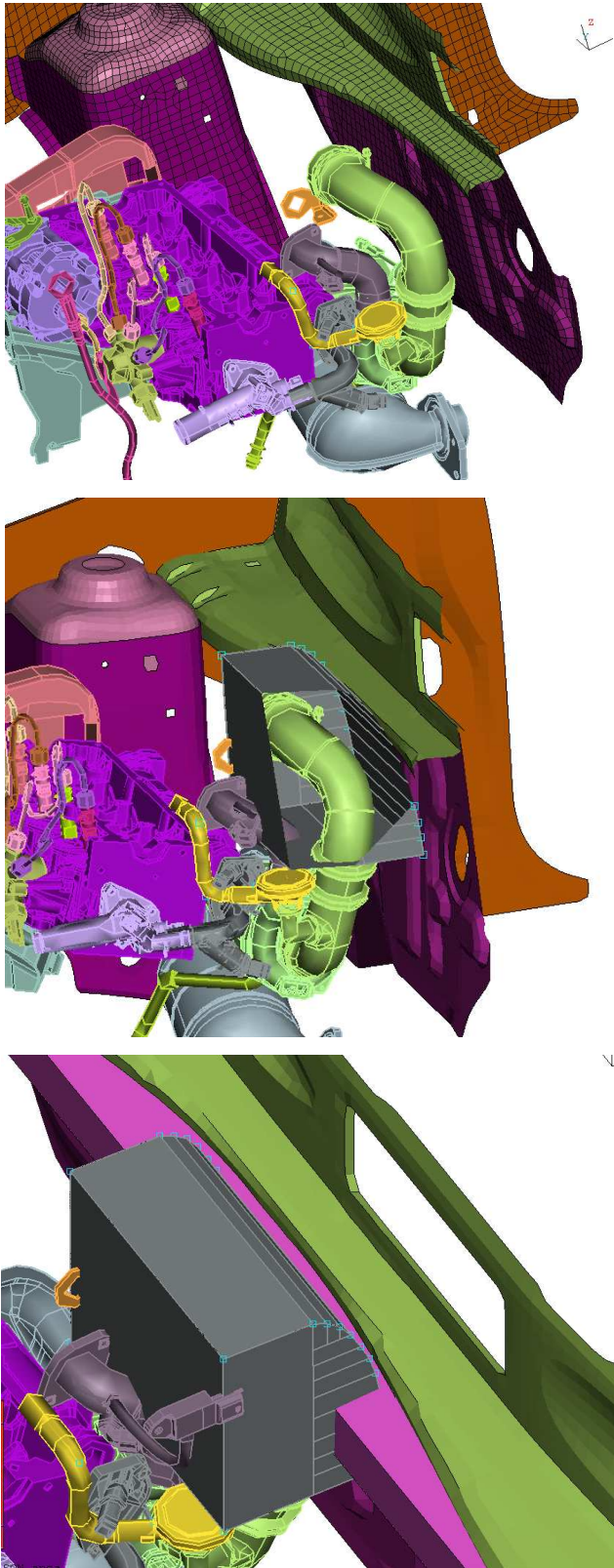
Figure 31. Process of volume allocation within CAE software
