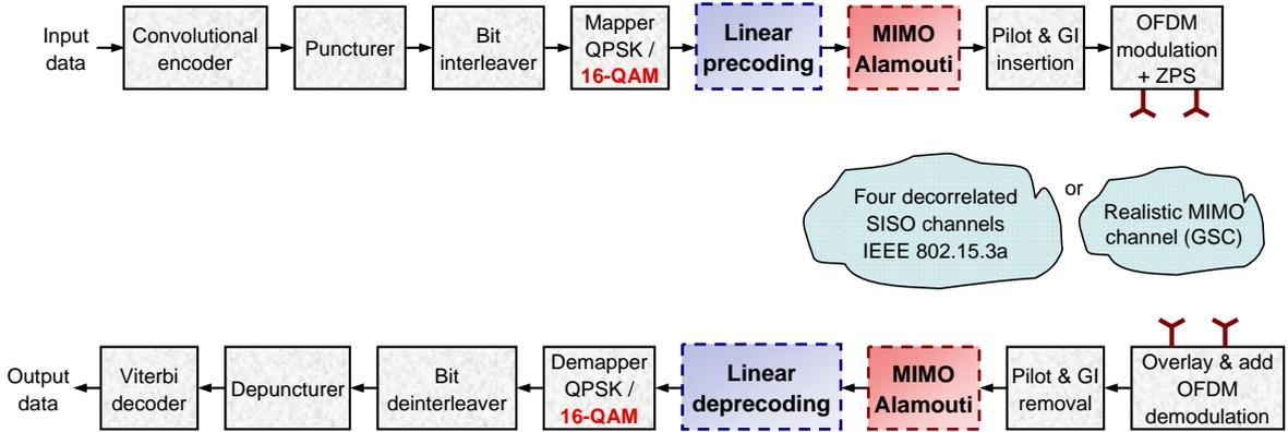
Figure 5.8: Simplified MIMO LP-OFDM UWB transmission system.
