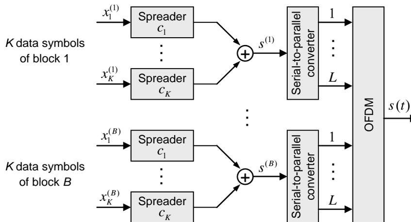
Figure 2.11: LP-OFDM transmitter for a single user.
