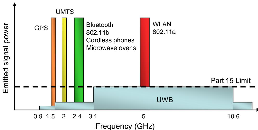
Figure 1.1: UWB spectrum overlaying existing narrowband systems.
