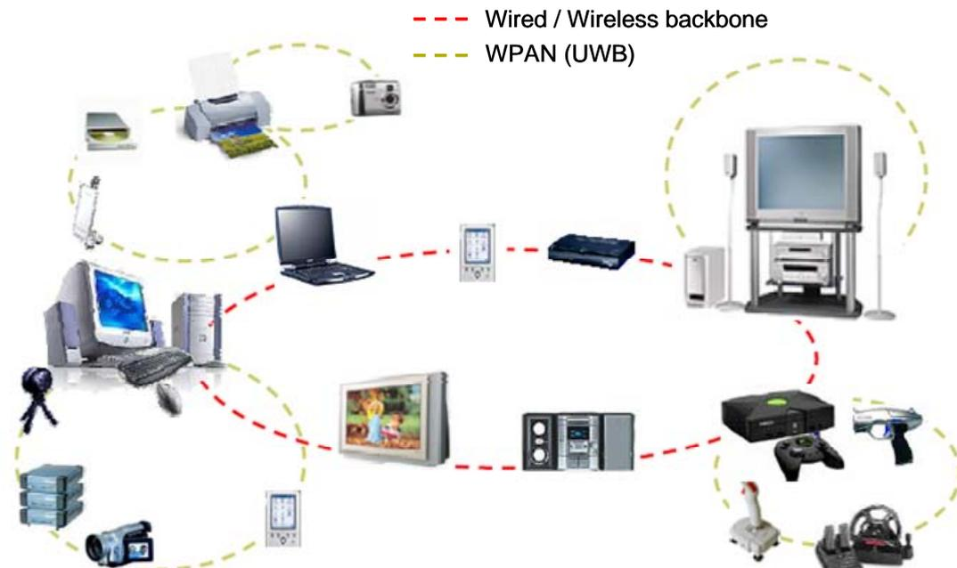
Figure 1.3: An example of a home networking setup using UWB technology.
