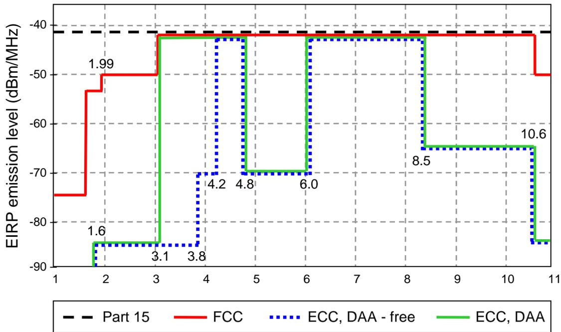
Figure 1.2: UWB spectrum mask for indoor communication systems.
