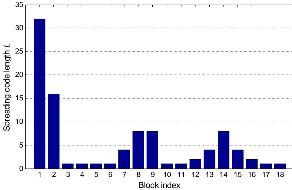
Figure 4.4: An example of the suboptimal code length configuration provided by the mean BER minimization algorithm for a given channel realization at  $E_b / N_0 = 8$  dB .
