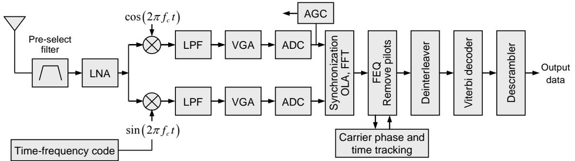
Figure 2.7: Receiver architecture for the MB-OFDM system.
