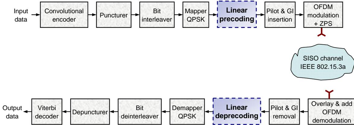
Figure 5.1: Simplified SISO LP-OFDM UWB transmission system.
