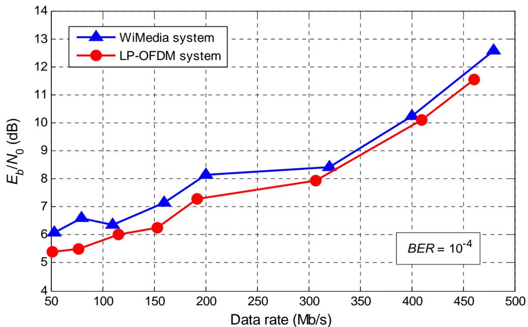
Figure 5.5: Required  $E_b / N_0$  to obtain  $BER = 10^{-4}$  at the output of the Viterbi decoder, for the different WiMedia and LP-OFDM data rates.
