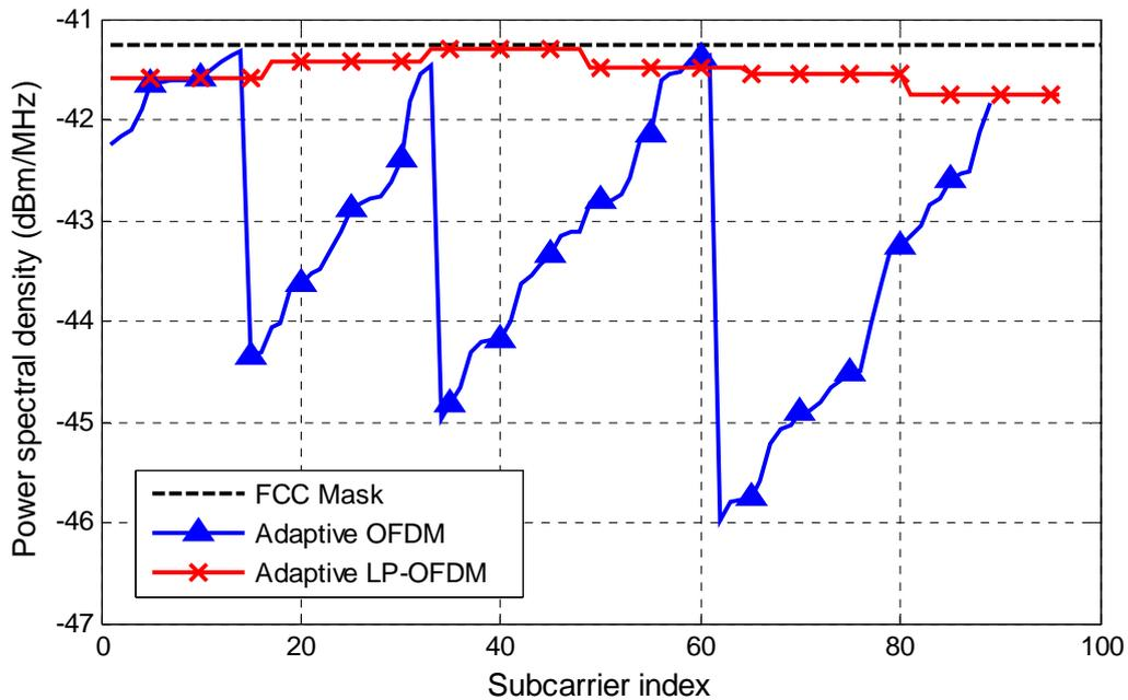
Figure 3.6: Effective transmitted power spectral density for the adaptive OFDM and LP-OFDM systems using variable constellation orders.
