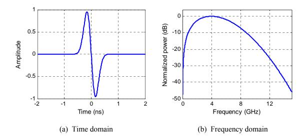
Figure 1.4: First-order Gaussian monocycle.
