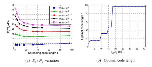
Figure 5.2: Spreading code length optimization in a LP-OFDM system without channel coding.
