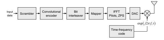
Figure 2.5: Transmitter architecture for the MB-OFDM system.
