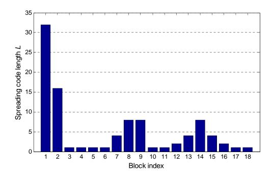
Figure 4.4: An example of the suboptimal code length configuration provided by the mean BER minimization algorithm for a given channel realization at  $E_b / N_0 = 8 \text{ dB}$ .
