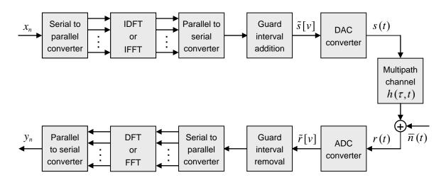
Figure 2.2: OFDM transmission system.
