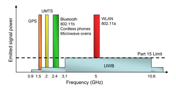
Figure 1.1: UWB spectrum overlaying existing narrowband systems.
