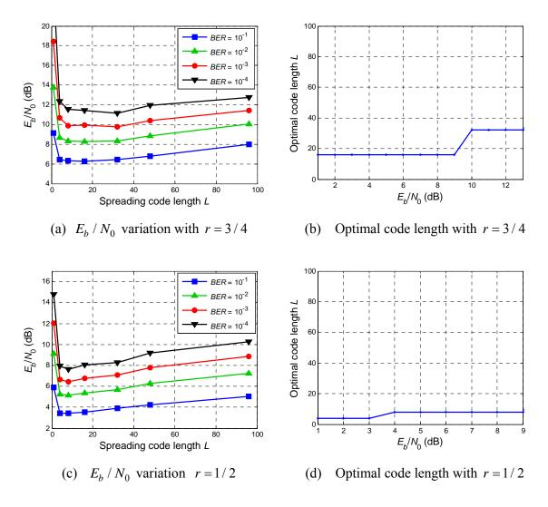
Figure 5.3: Spreading code length optimization for different channel coding rates in a global LP-OFDM system.
