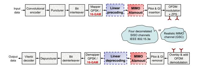
Figure 5.8: Simplified MIMO LP-OFDM UWB transmission system.
