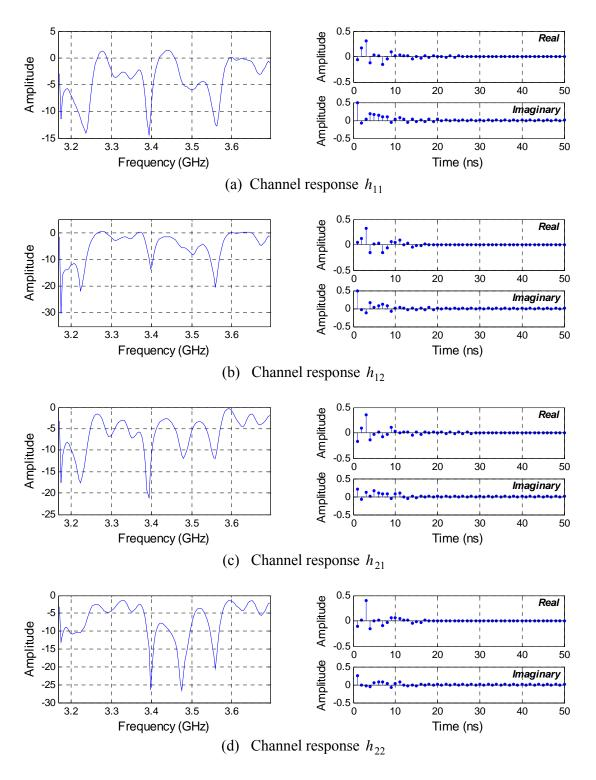
Figure 5.7: A typical channel realization of the proposed MIMO UWB channel model, with two transmit and two receive antennas, and an antennas spacing of d = 1 cm, presented in the frequency and time domains.
