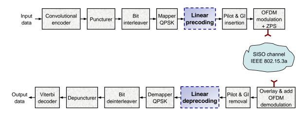
Figure 5.1: Simplified SISO LP-OFDM UWB transmission system.
