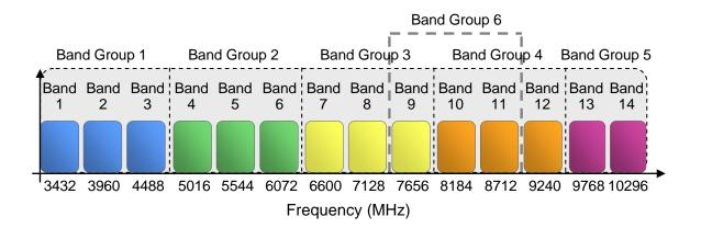
Figure 1.5: UWB spectrum bands in the MB-OFDM system.
