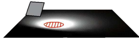
Figure 6: The C1 conjecture: the radiosity function has indefinite concavity everywhere, except over a convex area (hatched), where the radiosity function is concave.
