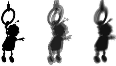
Figure 10: Combining several occlusion maps to compute soft shadows. Left: the occlusion map computed for a single sample. Center: the attenuation map computed using 4 samples. Right: the attenuation map computed using 64 samples.
