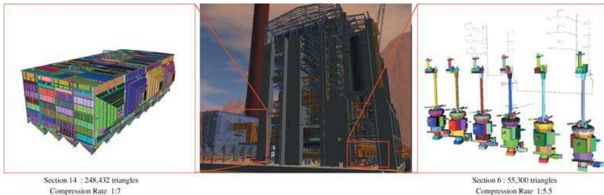
Fig. 12. Detecting symmetries and similarities between tiles created from a raw list of polygons allows us to compress geometric models in two ways: (1) by instancing similar tiles and (2) inside each symmetric tile, by instancing the part of the geometry which permits to reconstruct the whole tile. In such a big model as the powerplant (13 millions triangles), we achieve a compression ratio (ratio of geometry file size in X3D format) of 1:4.5. We show in this figure two subparts of the complete model. For each, we show the tiles computed by our heuristic (see Section 6.5) as well as the obtained compression ratio. The PowerPlant model is a courtesy of The Walkthru Project.
