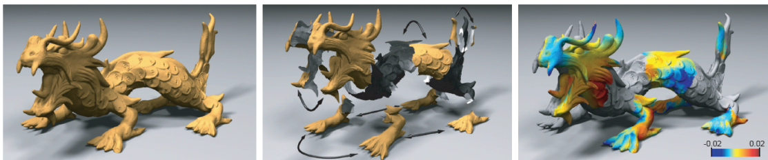
Figure 3.9: In [Mitra et al., 2006], the authors presented a technique to compute partial and approximate symmetries, based on a clustering in a well-chosen vector space.
