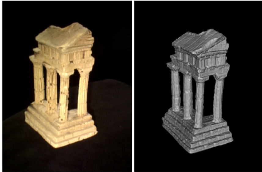
Figure 1.4: Reconstruction ( right ) with the method of [Goesele et al., 2006] of a temple and an input image ( left ) for comparison.
