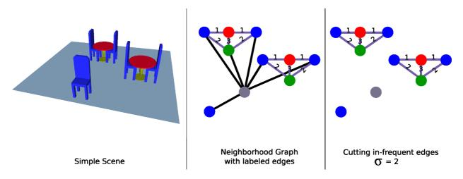
Figure 8.19: Left) A simple scene. Right) Its neighborhood graph. We affect to each edge a label with the property that two edges share the same label if the objects they define are congruent. In this example, we do not show the label of black edges as they appear only once in the scene.
