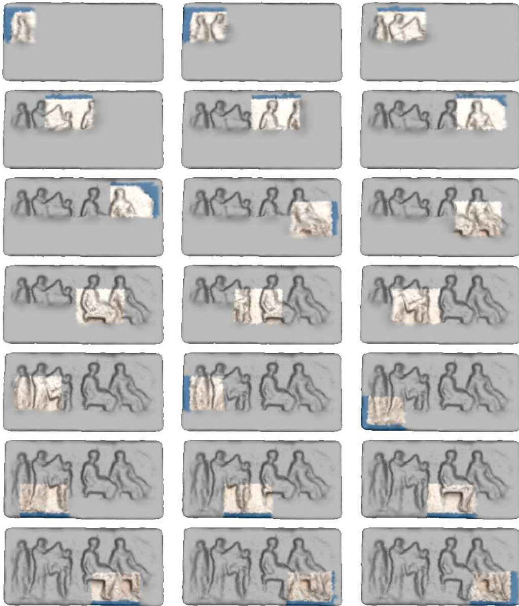
Figure 6.8: Parthenon reconstruction using 200 cameras and 21 clusters of cameras. We show partial reconstructions where parts of the surface are reconstructed using cameras belonging to one cluster at a time.
