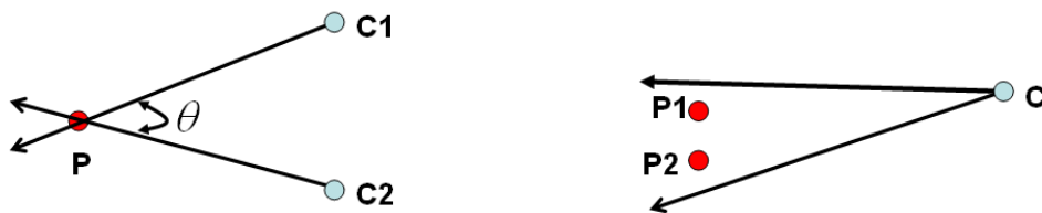
Figure 11.2: Left: Two projection rays intersecting to reconstruct a 3D point P . Right: Two 3D points P1 and P2 are lying between two consecutive projection rays.
