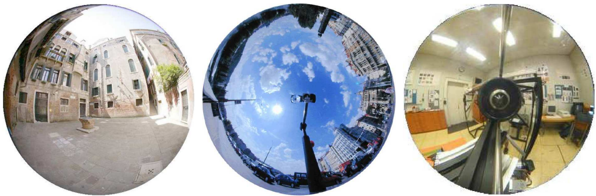
Figure 1.4: Omnidirectional images captured by three different cameras are shown: (a) image of a fisheye camera (b) image of a catadioptric camera using a hyperbolic mirror and a pinhole camera. (c) image of a catadioptric camera using a parabolic mirror and an orthographic camera.
