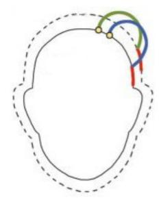
**Figure 5.8**: Hair volume is simulated using the multiple layer hulls method of [LK01]. Hairs with roots in higher positions collide with larger offsets of the head model (figure adapted from [LK01]).
