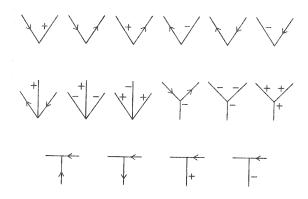
Figure 8.13: 16 junction types, adapted from Huffman
