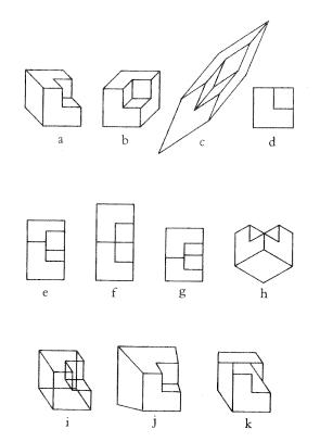
Figure 8.16: Which is the best representation of this cube with a missing corner? (a)
