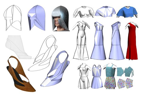
Figure 4.1: Developable helmet, shoe and garments generated from their sketched contours.
