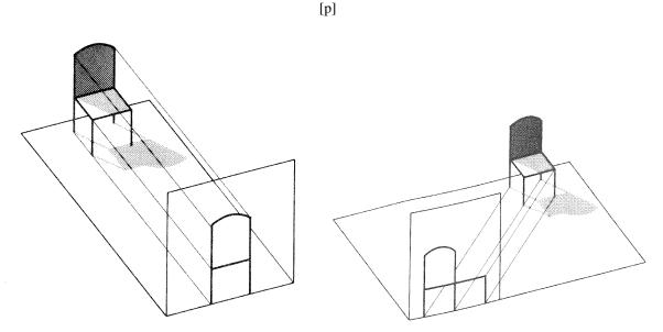
Figure 8.6: Orthogonal projection (left), Horizontal oblique projection (right)
