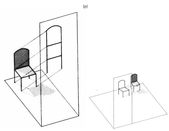
Figure 8.7: Vertical oblique projection (left), Oblique projection (right)
