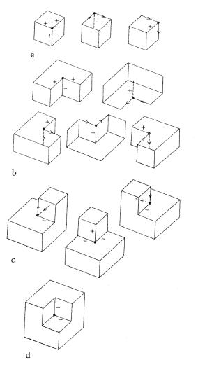
Figure 8.12: Huffmans 12 corner configurations
