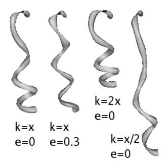
Figure 5.5: The physically-based hair strand is controlled by four main parameters: length, natural curliness, ellipticity and stiffness. Several strands hanging under the effect of gravity are depicted. All have the same length and natural curliness, but different values for the ellipticity e and the stiffness k. x = 1.6GPa.
