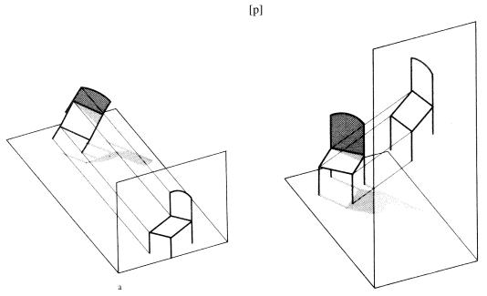
Figure 8.8: Isometric projection (left), Axonometric projection (right)
