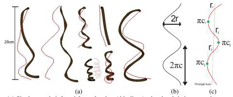
**Figure 5.6**: (a) Single strands inferred from sketches (thin lines): the sketch is interpreted as an example of the desired shape, our system generates similar, physically-based 3D strands (thick lines). (b) The orthogonal projection of a circular helix, and the measurements which can be made on it. (c) Inferring the length of a stroke using half helical segments.
