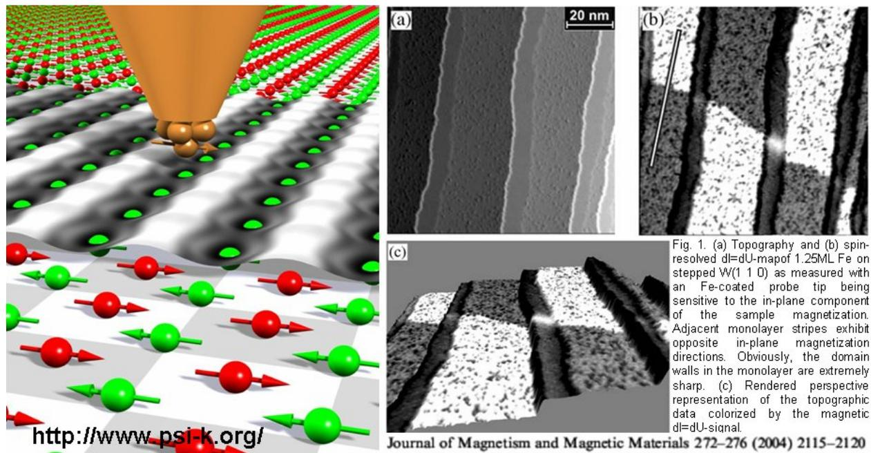
Fig. 1. (a) Topography and (b) spin-resolved  $dI=dU$ -map of 1.25 ML Fe on stepped W(1 1 0) as measured with an Fe-coated probe tip being sensitive to the in-plane component of the sample magnetization. Adjacent monolayer stripes exhibit opposite in-plane magnetization directions. Obviously, the domain walls in the monolayer are extremely sharp. (c) Rendered perspective representation of the topographic data colored by the magnetic  $dI=dU$ -signal.
