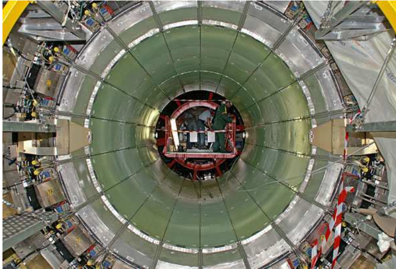
Figure 2.3: All barrel supermodules mounted in their final position inside the CMS hadron calorimeter.
