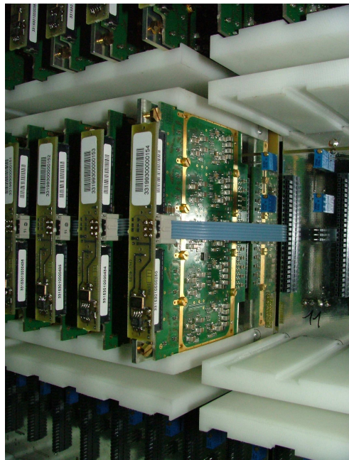
Figure 5.5: Left: The set-up of the burn-in system at IPN Lyon. Other 150 VFE cards can be plugged in the back of the system. Right: Detailed view of the plugged VFE cards.
