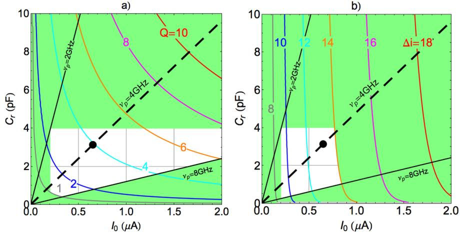
**Fig. 2.8.** Choice of readout oscillator parameters. a) Iso-Q curves (color lines) and iso- $\nu_p$  (black lines) in the  $I_0 - C_r$  plane at zero bias current. b) Iso- $\Delta i$  curves (color lines). The dash line indicates the chosen plasma frequency  $\nu_p = 4\text{GHz}$ . Green areas are discarded to avoid retrapping, to get small enough capacitor, a sufficiently low  $\nu_p$ , and a sufficient sensitivity. Black dot indicates our final target point
