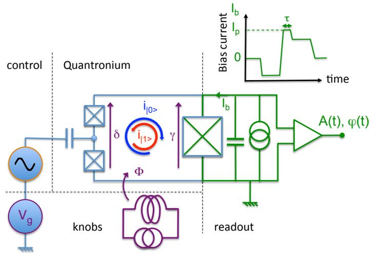
**Fig. 1.6.** Electrical scheme of the quantronium qubit. The qubit is in blue and the readout circuit in green. A large Josephson junction is inserted in the split CPB loop to serve as a threshold detector: a current pulse  $I_b(t)$  (top right) with a peak value  $I_p$  applied during a duration  $\tau$  induces the switching of the junction to a finite voltage with a probability that depends on the qubit state.
