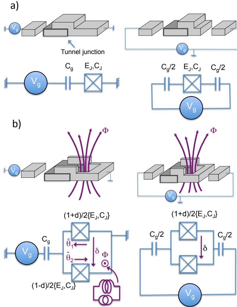
**Fig. 1.1.** Schematic representation and electrical schemes of the basic CPB (a) and split CPB (b), in its original version with one island and a reservoir (left) and in its symmetrized version (right).
