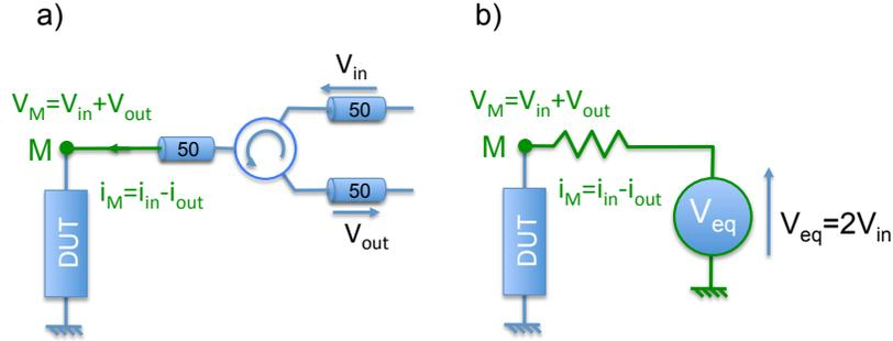
**Fig. F.2.** Schematic representation of circuit for microwave reflectometry measurement.
