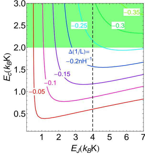
**Fig. 5.6.** Iso-amplitude of variation of  $1/L(N_g, \delta = \pi)$  as a function of  $E_J$  and  $E_C$  for  $d = 0.15$ . The green region indicates forbidden values of  $E_J$  and  $E_C$  in order to avoid poisoning. Our target design values are at the intersection of the dashed line and of the green border.
