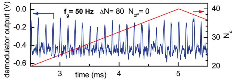
**Fig. 5.12.** Quadrature of the demodulated reflected signal (blue trace) when the gate charge is varied at low frequency (red trace). The periodic oscillations of the reflection coefficient result from the Bloch oscillations of the current-biased split cooper Pair Box during the linear ramps. Each period corresponds to a single Cooper pair injected in the box island.
