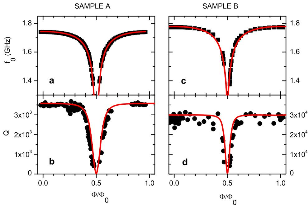
**Fig. 5** (Color online) (a, c) Measured resonance frequency  $f_0$  as a function of  $\Phi/\Phi_0$  (squares) for samples A and B, respectively, and fit according to (7) (solid line). (b, d) Measured quality factor  $Q$  (disks) as a function of  $\Phi/\Phi_0$ . The solid line is calculated according to the model (see text) for a temperature  $T = 60$  mK
