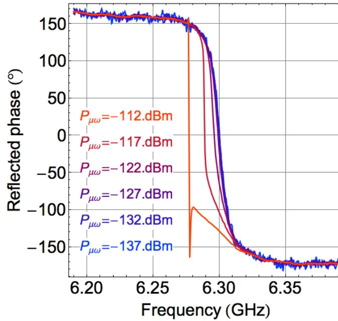
**Fig. 4.12.** Resonator measurements with a Vector Network Analyzer. Phase of the reflected signal as a function of the microwave frequency  $\omega_{rf}$  for various input powers. At high power, the resonance curve shifts towards low frequency and sharpens, indicating the bifurcation phenomenon.
