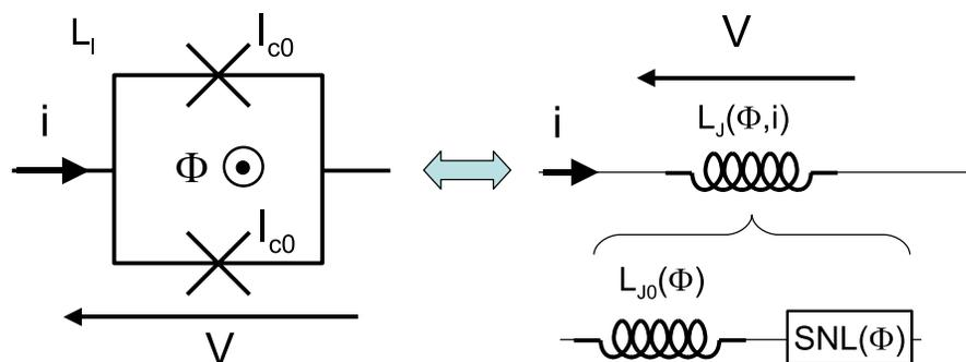
**Fig. 2** A DC SQUID with two junctions of critical current  $I_{c0}$  and loop inductance  $L_l$ , biased by a magnetic flux  $\Phi$  and by a current  $i$ , is equivalent to a lumped flux-dependent non-linear inductance  $L_J(\Phi, i)$  that can be decomposed in an inductance  $L_{J0}(\Phi)$  and a non-linear element  $SNL(\Phi)$  in series
