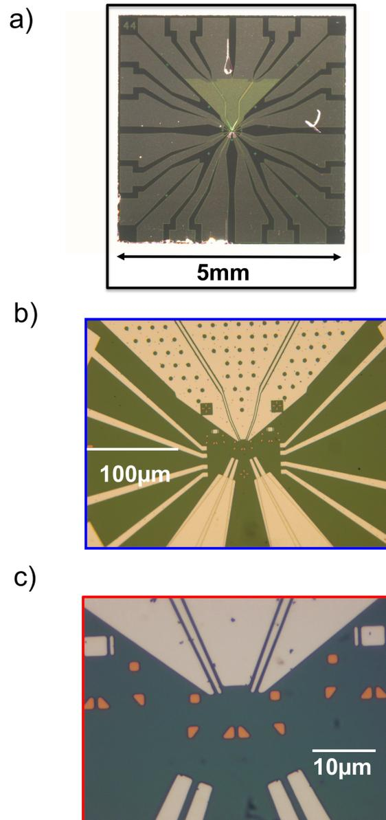
**Fig. 2.14.** Optical micrographies of a quantroswap chip before e-beam lithography. One can see the whole chip (a), the readout capacitor (bottom structure) and the  $100 \times 100 \mu\text{m}^2$  central area for e-beam lithography (b), as well as the central part with the gates (top electrodes), the readout leads (bottom electrodes), and the quasiparticles (small yellow pads)
