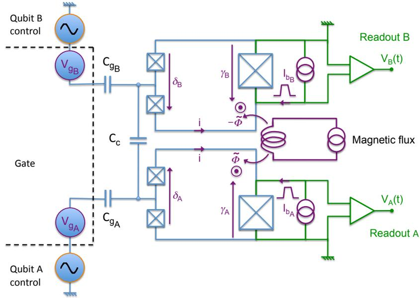
**Fig. 1.10.** Simplified diagram of the Quantroswap circuit with 2 quantroniums whose islands are capacitively coupled. Each qubit has its own gate and readout. The fluxes through the loops are applied using the same coil and have consequently opposite signs, considering the orientation of the different phases, voltages and loop current.
