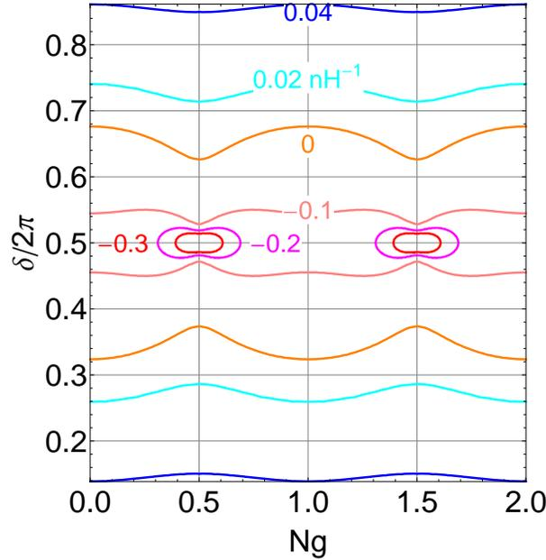
**Fig. 5.3.** Iso-inverse inductance of the split CPB as a function of its working point  $(N_g, \delta)$  for  $E_J = 2k_B K$ ,  $E_C = 1k_B K$  and  $d = 0.05$ . This inductance is 1-periodic in  $N_g$ , and its maximal modulation in  $N_g$  occurs at  $\delta = \pi$ .
