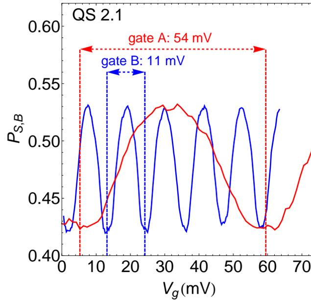
**Fig. 3.5.** Measurement of the DC gate capacitances in sample QS 2.1. The two curves show the modulation of the switching probability  $P_S$  of qubit B (in the ground state) as a function of the gate voltages  $V_{g_B}$  (red) and  $V_{g_A}$  (blue). From the voltage periodicity, one can determine the gate capacitances (29 aF and 6 aF), and the parasitic crosstalk (20%).
