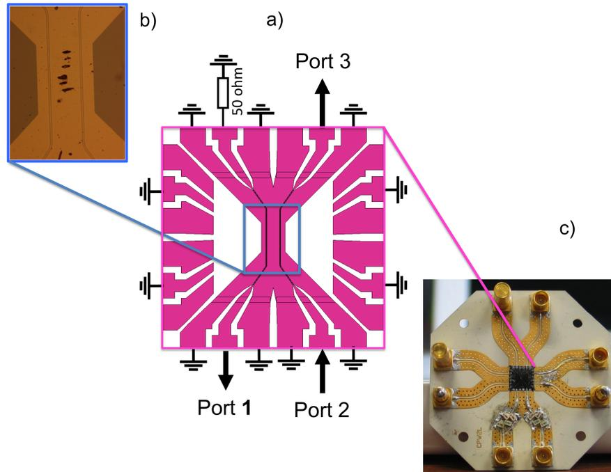
**Fig. E.1.** Geometry of the special chip used in the PCB characterization (quantroswap experiment). a) Drawing of the chip with its two  $50\Omega$  niobium microwave coplanar waveguides. Arrows indicates the different ports for the S parameters. b) Detailed optical micrograph of the central part. c) Overall view of the PCB with the surface mounted filters of the readout lines.
