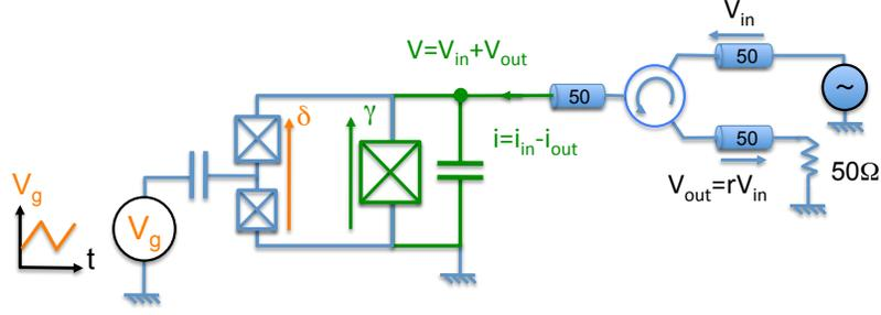
**Fig. 5.4.** Electrical scheme of the Blochonium circuit. A  $50 \Omega$  source applies an incoming wave of amplitude  $V_{in}$  to a quantonium-like sample. This wave is reflected on the Blochonium oscillator and propagates through a circulator to a  $50 \Omega$  amplifier ( $50 \Omega$  resistor on the figure).
