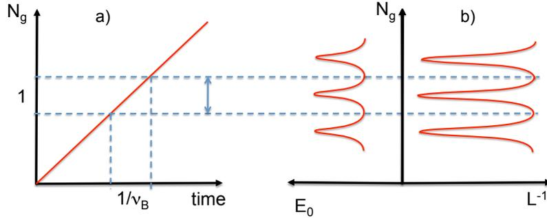
**Fig. 5.2.** Principle of the current to frequency conversion with a Cooper pair box. a) Linear evolution of  $N_g(t)$ . b) Ground state energy band (left) and its second derivative  $L^{-1}$  with respect to  $\delta$  (right) as a function of  $N_g$ .
