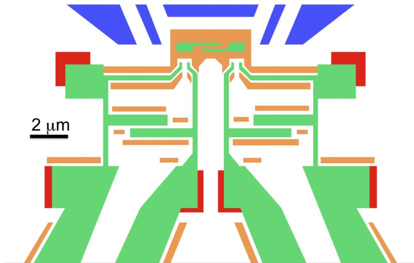
**Fig. 2.16.** E-beam exposure pattern of the central part of the quantroswap circuit. Green areas correspond to openings through the PMMA resist, that define the various quantroswap electrodes, whereas orange elements correspond to lower exposure dose aiming at increasing the undercut below the suspended mask. Blue and red areas represent the optically pre-fabricated gates and quasiparticles traps.
