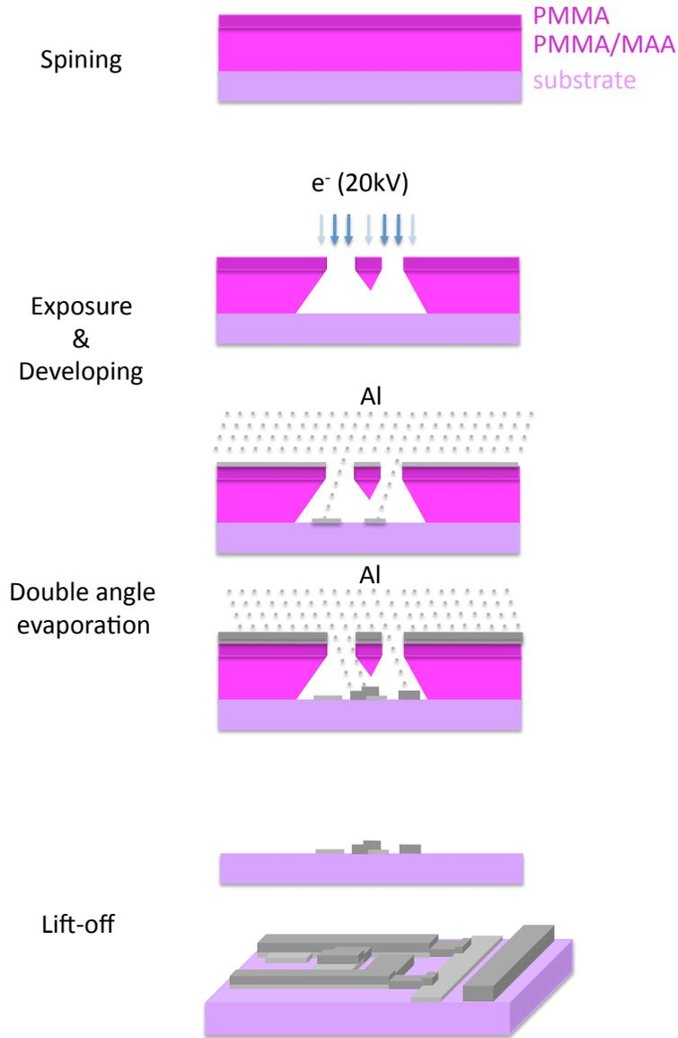
**Fig. C.4.** Electronic lithography process. PMMA-MMA and PMMA-MAA resist (pink) are spinned. Then specific part are exposed by steering on the desired pattern electrons. Aluminum is then evaporated a first time at a first angle, then aluminum is oxidized to form a thin layer of insulator, and a second layer of aluminum is deposited at a different angle. Finally the resist is removed. Overlapping layers form the Josephson junctions.
