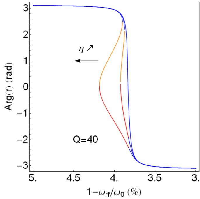
**Fig. F.6.** Calculated phase of the reflection coefficient  $r$  in the linear and non-linear regimes from the solutions  $\gamma_a$  plotted in Fig. F.5. The phase are multi-valued for certain values  $\eta$  and  $\omega_{rf}$ .
