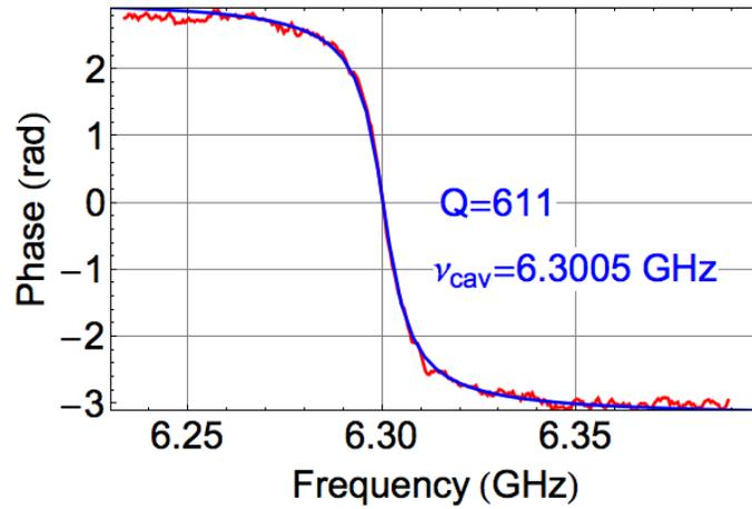
**Fig. 4.13.** Determination of the resonance frequency  $\nu_{cav}$  and quality factor  $Q$  of the resonator. Note that the resonance frequency is changed by about 2.5 MHz compared to fig. 4.11 due to the change of the working point of the qubit. Here  $\omega_{ge} \ll \omega_{cav}$ .
