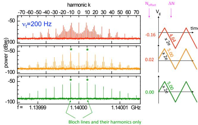
**Fig. 5.13.** Spectra of a reflected signal at 1.14 GHz for different triangular gate voltages (see pictograms on the right) at frequency  $\nu_g=200$  Hz. These spectra consist in peaks at the different harmonics at frequency  $i \times \nu_g$ . When  $N_{g0}$  and  $\Delta N_g$  are tuned to integer values only peaks at the Bloch frequency and its multiple  $\nu_B = 2\Delta N_g \nu_g$  remain (see bottom panel).
