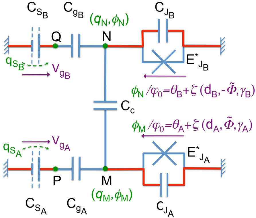
**Fig. 1.11.** Model electrical circuit of the quantroswap: the chosen spanning tree leading to the four M,N,P,Q nodes is indicated in red. The two couples  $\{q_M, \phi_M\}$   $\{q_N, \phi_N\}$  of conjugated node variables chosen as the degrees of freedom of the system are shown. The voltage sources  $V_{g_{A,B}}$  are modeled by infinite capacitor  $C_{S_{A,B}}$  having delivered a charge  $q_{S_{A,B}}$ .
