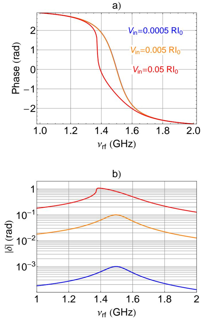
**Fig. 5.7.** Response of the Blochonium oscillator to microwave excitation as a function of the probe signal frequency for three drive amplitudes  $|2V_{\text{in}}/(RI_0)| = 0.001$  (blue), 0.01 (orange) and 0.1 (red): phase of the reflected signal (a) and amplitude  $\gamma_a$  of oscillations (b) for  $\nu_p = 1.5$  GHz and  $Q = 10$ .
