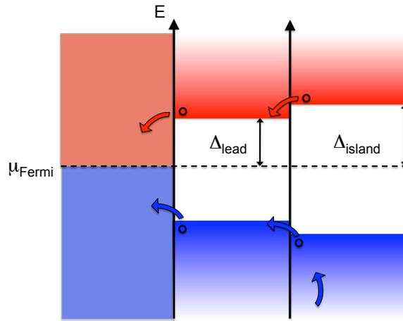
**Fig. 2.13.** Removing quasiparticles from the quantronium islands. The graph represents the quasiparticle density of state in a non-superconducting electrode (left), a thick superconducting Al lead (center), and thin Al island (right). Electron-like (red) and hole-like (blue) quasiparticles in the superconducting island (right) tend to tunnel to the lead and then to diffuse to the normal metal, where they get thermalized and trapped.
