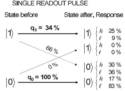
FIG. 4. Readout outputs and qubit state evolution in a measurement by a single readout pulse. The kets  $|\psi=0,1\rangle$  indicate the qubit state before (left) and after (right) the measurement. The arrows and their associated probabilities correspond to the different possible qubit evolutions. The QND fractions are indicated in bold. The different readout responses for each different scenario are indicated on the right with their probabilities.
