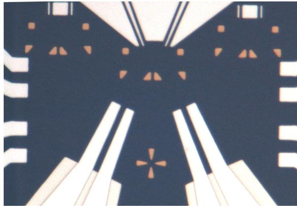
**Fig. C.3.** Micrographies of the central part of the quantroswap chip after three optical lithography steps. a) Optical micrography. Bottom aluminum electrodes (bottom of the Figure), then gold pads (yellow), and finally top aluminum layer were deposited successively. Gold crosses are used for further alignment in e-beam lithography. b) SEM micrography showing both the optical and e-beam fabricated electrodes. The lateral size of the optically made quantronium gates is indicated.
