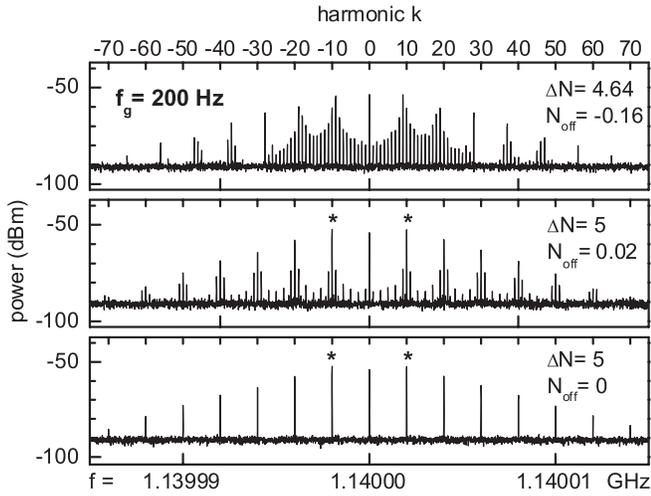
FIG. 3. Spectrum of a reflected cw signal at 1.14 GHz for different triangular wave gate modulation patterns, at frequency  $f_g = 200$  Hz. The spectrum consists of sidebands shifted by  $kf_g$  from the carrier. Progressive tuning of the amplitude  $\Delta N$  and of the offset  $N_{\text{off}}$  yields a spectrum consisting only of Bloch lines shifted from the carrier by a multiple of  $f_B = 2\Delta N f_g$ . The Bloch lines of order 1 ( $k = \pm 2\Delta N$ ) are marked by an asterisk.
