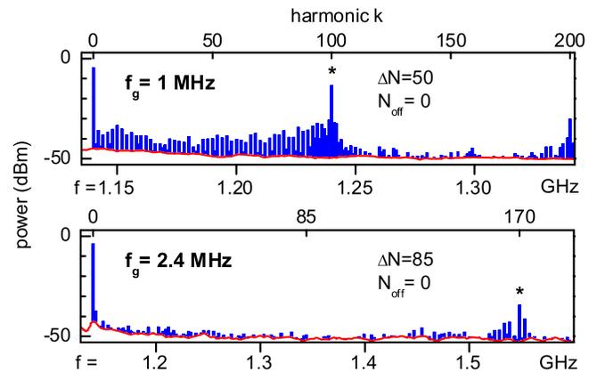
FIG. 5 (color online). Amplitude of the sidebands at positive harmonics (top scale) of the gate frequency  $f_g$ . Top panel:  $\Delta N = 50$ ,  $f_g = 1$  MHz ( $I = 32$  pA,  $f_B = 100$  MHz); bottom panel:  $\Delta N = 85$ ,  $f_g = 2.4$  MHz ( $I = 130$  pA,  $f_B = 408$  MHz). The Bloch line of order 1 is marked by an asterisk. The continuous line is the noise level. We attribute the presence of non-Bloch lines to the imperfections in the gate signal, and to charge noise.
