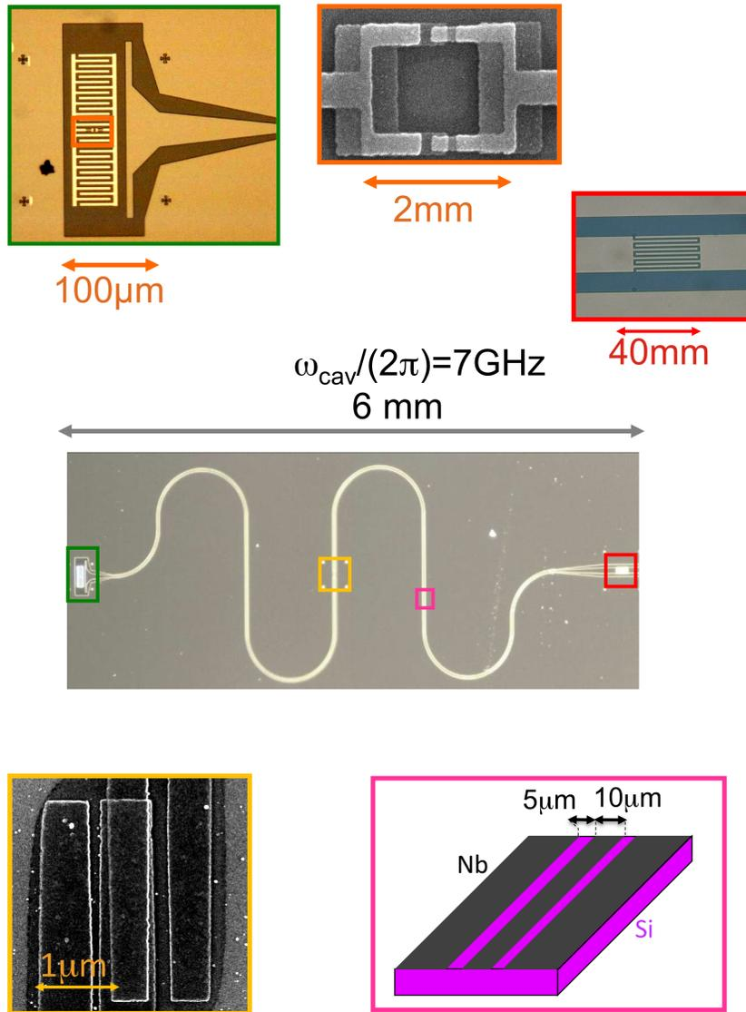
**Fig. 4.9.** Pictures of the main circuit elements. In the center, the Coplanar Waveguide resonator. At its left side (green) is placed the transmon (top left), while at its right side, it is connected to  $50\ \Omega$  line through an interdigitated capacitor (red) (top right). In the middle of the resonator (yellow), a Josephson junction is inserted in the inner conductor.
