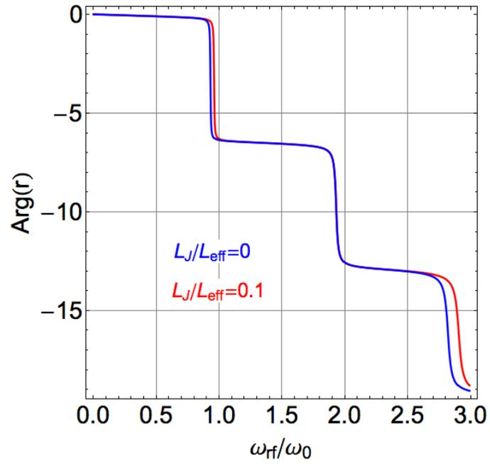
**Fig. F.4.** Calculated phases of the reflected signal in the linear regime as a function of the drive frequency  $\omega_{rf}$  for two values of the Josephson inductance inserted at the center of a  $\lambda/2$  resonator. The resonance frequency of the second harmonic ( $\omega_{rf} = 2\omega_0$ ) is not modified by the presence of the Josephson junction at the center of the resonator as this point corresponds to a node of the current for even harmonics of  $\omega_0$ .
