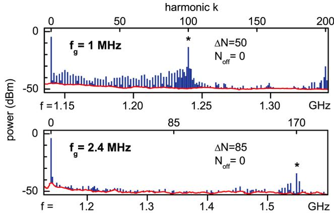
**Fig. 5.15.** Amplitudes of the harmonics of  $\nu_B$ . Top:  $N_{g0} = 0$ ,  $\Delta N_g = 50$ , and  $\nu_g = 1$  MHz. Bottom:  $N_{g0} = 0$ ,  $\Delta N_g = 85$ , and  $\nu_g = 2.4$  MHz. The Bloch lines of order 1 are marked with an asterisk and correspond to Bloch frequency of 100 MHz = 32 pA and 408 MHz = 130 pA.
