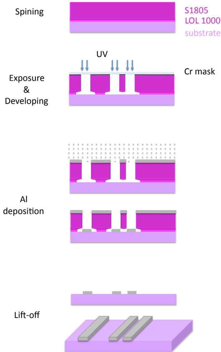
**Fig. C.1.** Illustration of the submicron optical lithography process developed during this thesis work. LOL1000 and S1805 resist (pink) are first spun on a Si-SiO<sub>2</sub> or sapphire 2-inch wafer. In a second step, the wafer is exposed to a monochromatic UV light (i line) through a Cr-quartz 3-inch mask. The exposed resist is developed by immersion in MF319. Then metal is evaporated in an electron gun evaporator. Finally the mask is lifted off.
