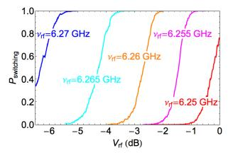
Fig. 4.15. Switching probabilities  $P_S$  as a function of the microwave signal power for different values of the microwave frequency  $\omega_{rf}$ . The microwave pulse has a plateau duration of 150 ns, and a latching duration of 400 ns.
