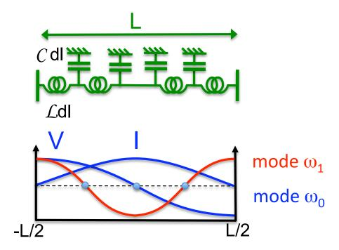
Fig. 4.3. Schematic representation of a distributed microwave resonator of length L.
