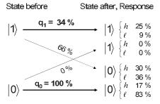
FIG. 4. Readout outputs and qubit state evolution in a measurement by a single readout pulse. The kets  $|\psi=0,1\rangle$  indicate the qubit state before (left) and after (right) the measurement. The arrows and their associated probabilities correspond to the different possible qubit evolutions. The QND fractions are indicated in bold. The different readout responses for each different scenario are indicated on the right with their probabilities.
