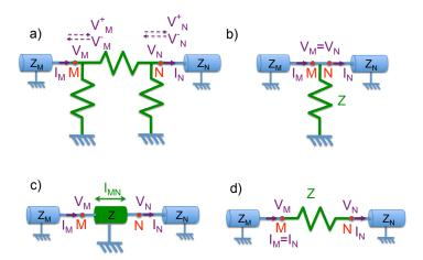
**Fig. F.1.** Schematic representation of circuits a) General representation of a electrical component (green) connected to two points M and N, and the associated voltages and currents. b) Case where the component is a discrete impedance Z connected to ground. c) Case where the element is transmission line of impedance Z and length l. d) Case where M and N are connected through a discrete impedance Z.
