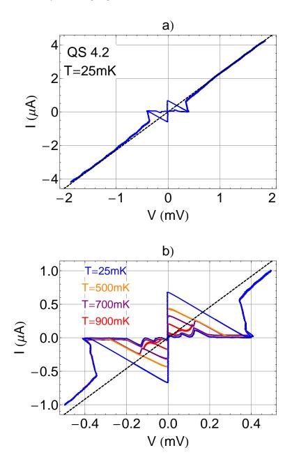
Fig. 3.2. I-V curves of sample QS 4.2 at different scales and different temperatures during cooling. a) Large scale IV curve whose slope gives a 436  $\Omega$  tunnel resistance. b) IV curves at a smaller scale and at different temperatures showing the superconducting gap as well as subgap structures attributed to dissipative resonances in the environment at high-frequency.
