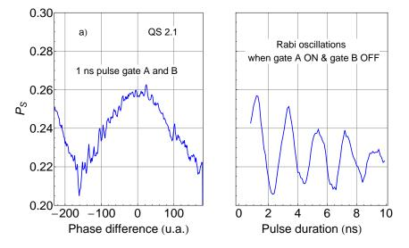
**Fig. 3.14.** Calibration of the phase shift between the two gate lines. a) Switching probability as a function of the dephasing due to the phase shifter when a microwave pulse is applied on both gates. b) Reference contrast (Rabi oscillations) on the same qubit with only one microwave applied.
