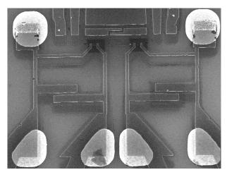
Fig. C.5. SEM image of central part of quantroswap circuit.
