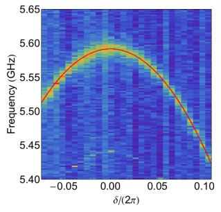
**Fig. 4.16.** Spectroscopy of the transition  $|g\rangle - |e\rangle$ . The spectroscopy of the transition  $|e\rangle - |f\rangle$  gave a difference  $\omega_{ge} - \omega_{ef} = 300$  MHz, yielding  $E_C = 0.05$ K. One can thus fit (red) the spectroscopy with  $E_J = 0.698$ K. The two photon transition  $|g\rangle \rightarrow |f\rangle$  is visible in the bottom of the figure.
