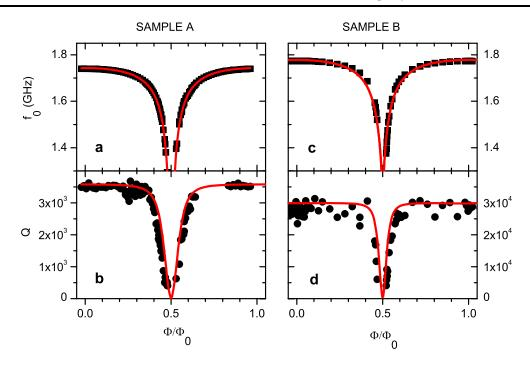
**Fig. 5** (Color online) (**a**, **c**) Measured resonance frequency  $f_0$  as a function of  $\Phi/\Phi_0$  (squares) for samples A and B, respectively, and fit according to (7) (solid line). (**b**, **d**) Measured quality factor Q (disks) as a function of  $\Phi/\Phi_0$ . The solid line is calculated according to the model (see text) for a temperature T = 60 mK
