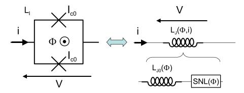
Fig. 2 A DC SQUID with two junctions of critical current  $I_{c0}$  and loop inductance  $L_l$ , biased by a magnetic flux  $\Phi$  and by a current i, is equivalent to a lumped flux-dependent non-linear inductance  $L_J(\Phi,i)$  that can be decomposed in an inductance  $L_{J0}(\Phi)$  and a non-linear element SNL( $\Phi$ ) in series
