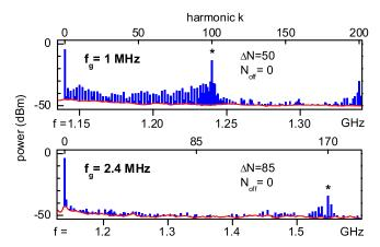
FIG. 5 (color online). Amplitude of the sidebands at positive harmonics (top scale) of the gate frequency  $f_g$ . Top panel:  $\Delta N = 50$ ,  $f_g = 1$  MHz (I = 32 pA,  $f_B = 100$  MHz); bottom panel:  $\Delta N = 85$ ,  $f_g = 2.4$  MHz (I = 130 pA,  $f_B = 408$  MHz). The Bloch line of order 1 is marked by an asterisk. The continuous line is the noise level. We attribute the presence of non-Bloch lines to the imperfections in the gate signal, and to charge noise.
