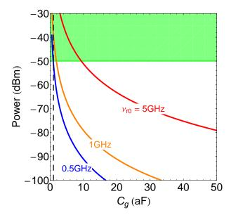
Fig. 2.5. Iso-values of the Rabi frequency as a function of gate capacitance  $C_g$  and of the microwave power applied to the gate for the selected values  $E_J=0.51~{\rm K}$   $E_C=0.97~{\rm K}$ . The green area corresponds to a gate power higher than available. Dashed vertical line indicates the minimal value for  $C_g$  in order to apply a  $\pi$  pulse in 1ns.
