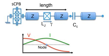
**Fig. 4.6.** Cavity Josephson Bifurcation Amplifier based dispersive readout scheme. A transmon is capacitively coupled to a microwave cavity resonator. A Josephson junction is inserted at the antinode of the magnetic field (and current), making the resonator non-linear.
