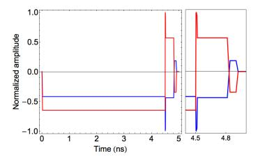
Fig. 3.15. Time dependence of the bias signals (unscaled) applied to readout A (blue) and readout B (red) for achieving the resonance condition, and for performing the readout.
