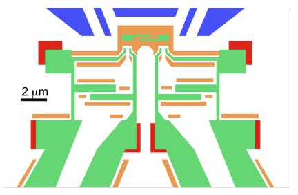
Fig. 2.16. E-beam exposure pattern of the central part of the quantroswap circuit. Green areas correspond to openings though the PMMA resist, that define the various quantroswap electrodes, whereas orange elements corresponds to lower exposure dose aiming at increasing the undercut below the suspended mask. Blue and red areas represent the optically pre-fabricated gates and quasiparticles traps.
