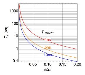
**Fig. 2.10.** Dephasing time  $T_{\varphi,SWAP}$  of a superposition  $\alpha |\Psi_1\rangle + \beta |\Psi_2\rangle$  with respect to the phase  $\delta$  for different swapping time  $T_{SWAP} = 1, 2, 10$  ns.
