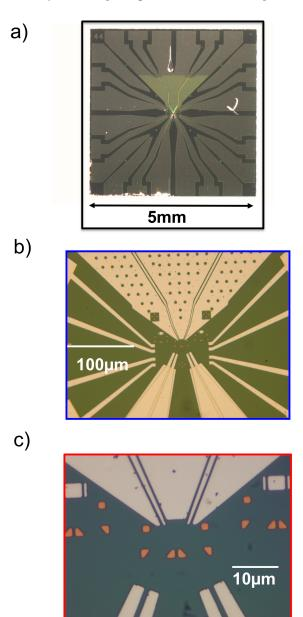
Fig. 2.14. Optical micrographies of a quantroswap chip before e-beam lithography. One can see the whole chip (a), the readout capacitor (bottom structure) and the  $100\times100\mu\text{m}^2$  central area for e-beam lithography (b), as well as the central part with the gates (top electrodes), the readout leads (bottom electrodes), and the quasiparticles (small yellow pads)
