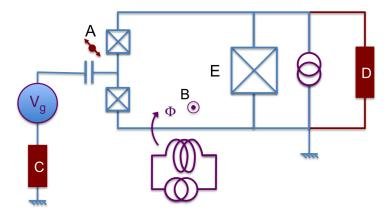
Fig. 1.8. Main decoherence sources in a quantronium device. Noise in  $N_g$  is generated by charged two-level fluctuators (A) in the vicinity of the island and by voltage fluctuations of series impedance (C) in the gate line. Noise in  $\delta$  is generated by fluctuations in the flux  $\phi$  (B), by current fluctuations in the finite impedance (D) of the readout bias source. Noise in  $E_J$  is induced by critical current fluctuations of the CPB junctions (E).
