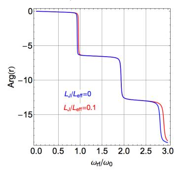
Fig. F.4. Calculated phases of the reflected signal in the linear regime as a function the drive frequency  $\omega_{rf}$  for two value of the Josephson inductance inserted at the center of a  $\lambda/2$  resonator. The resonance frequency of the second harmonic ( $\omega_{rf}=2\omega_0$ ) is not modified by the presence of the Josephson junction at the center of the resonator as this point corresponds to a node of the current for even harmonics of  $\omega_0$ .
