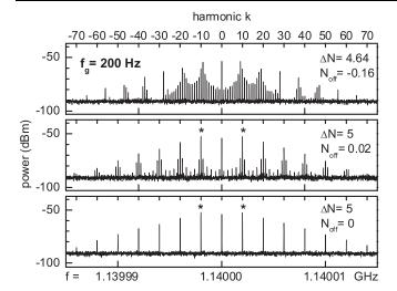
FIG. 3. Spectrum of a reflected cw signal at 1.14 GHz for different triangular wave gate modulation patterns, at frequency  $f_g = 200$  Hz. The spectrum consists of sidebands shifted by  $kf_g$  from the carrier. Progressive tuning of the amplitude  $\Delta N$  and of the offset  $N_{\rm off}$  yields a spectrum consisting only of Bloch lines shifted from the carrier by a multiple of  $f_B = 2\Delta N f_g$ . The Bloch lines of order 1 ( $k = \pm 2\Delta N$ ) are marked by an asterisk.
