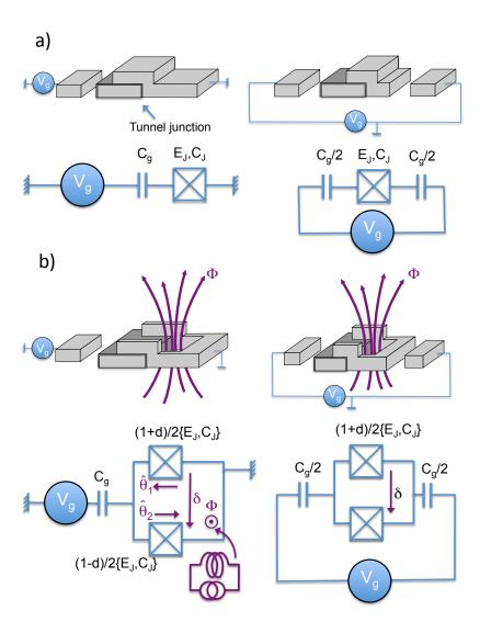
**Fig. 1.1.** Schematic representation and electrical schemes of the basic CPB (a) and split CPB (b), in its original version with one island and a reservoir (left) and in its symmetrized version (right).
