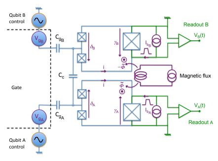
Fig. 1.10. Simplified diagram of the Quantroswap circuit with 2 quantroniums whose islands are capactively coupled. Each qubit has its own gate and readout. The fluxes through the loops are applied using the same coil and have consequently opposite signs, considering the orientation of the different phases, voltages and loop current.
