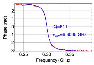
Fig. 4.13. Determination of the resonance frequency  $\nu_{cav}$  and quality factor Q of the resonator. Note that the resonance frequency is changed by about 2.5 MHz compared to fig. 4.11 due to the change of the working point of the qubit. Here  $\omega_{ge} << \omega_{cav}$ .
