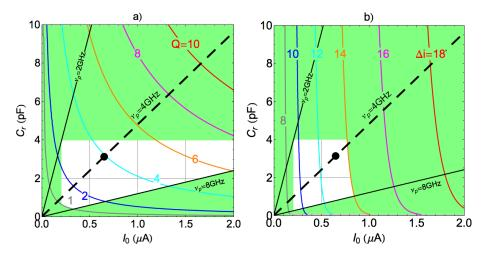
Fig. 2.8. Choice of readout oscillator parameters. a) Iso-Q curves (color lines) and iso- $\nu_p$  (black lines) in the  $I_0-C_r$  plane at zero bias current. b) Iso- $\Delta i$  curves (color lines). The dash line indicates the chosen plasma frequency  $\nu_p=4$  GHz. Green areas are discarded to avoid retrapping, to get small enough capacitor, a sufficiently low  $\nu_p$ , and a sufficient sensitivity. Black dot indicates our final target point
