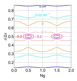
**Fig. 5.3.** Iso-inverse inductance of the split CPB as a function of its working point  $(N_g,\delta)$  for  $E_J=2k_BK$ ,  $E_C=1k_BK$  and d=0.05. This inductance is 1-periodic in  $N_g$ , and its maximal modulation in  $N_g$  occurs at  $\delta=\pi$ .
