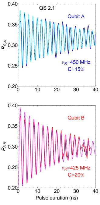
Fig. 3.12. Determination of the readout sensitivity using Rabi oscillations for both qubits. The lines are fit curves. The measured contrast and switching probabilities are used to calculated the expected switching probabilities in Fig. 3.16.
