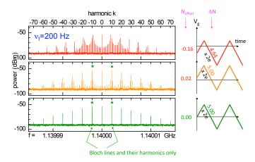
Fig. 5.13. Spectra of a reflected signal at 1.14 GHz for different triangular gate voltages (see pictograms on the right) at frequency  $\nu_g$ =200 Hz. These spectra consist in peaks at the different harmonics at frequency i× $\nu_g$ . When  $N_{g_0}$  and  $\Delta N_g$  are tuned to integer values only peaks at the Bloch frequency and its multiple  $\nu_B = 2\Delta N_g \nu_g$  remain (see bottom panel).
