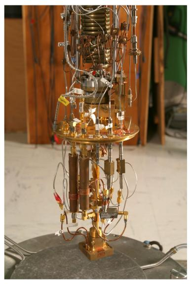
$\bf Fig.~2.19.$  Picture of the 20 mK to 600 mK stage of the experiment with the complete wiring.
