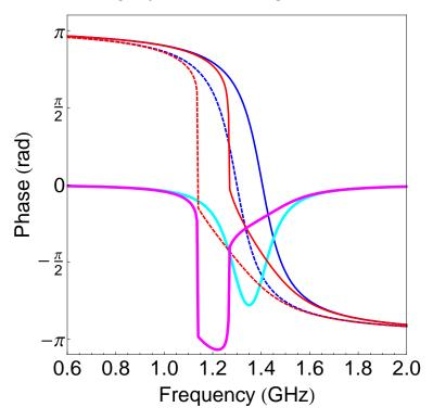
Fig. 5.8. Gate charge induced phase modulation of the Blochonium for  $\nu_p=1.5$  GHz,  $Q=10,\ E_J=4$  K,  $E_C=2$  K, and d=0.15. Thin lines are absolute phases of the reflected signal as a function of the probe signal frequency for two amplitudes  $|2V_{\rm in}/(RI_0)|=0.001$  (blue) and 0.1 (red), and for  $N_g=0$  (solid) and 1/2 (dashed). Bold lines are the corresponding differences between  $N_g=0$  and 1/2 for  $|2V_{\rm in}/(RI_0)|=0.001$  (cyan) and 0.1 (magenta).
