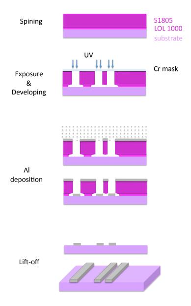
**Fig. C.1.** Illustration of the submicron optical lithography process developed during this thesis work. LOL1000 and S1805 resist (pink) are first spun on a Si-Si0<sub>2</sub> or sapphire 2-inch wafer. In a second step, the wafer is exposed to a monochromatic UV light (i line) trough a Cr-quartz 3-inch mask. The exposed resist is developed by immersion in MF319. Then metal is evaporated in an electron gun evaporator. Finally the mask is lifted off.
