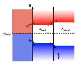
Fig. 2.13. Removing quasiparticles from the quantronium islands. The graph represents the quasiparticle density of state in a non-superconducting electrode (left), a thick superconducting Al lead (center), and thin Al island (right). Electron-like (red) and hole-like (blue) quasiparticles in the superconducting island (right) tend to tunnel to the lead and then to diffuse to the normal metal, where they get thermalized and trapped.
