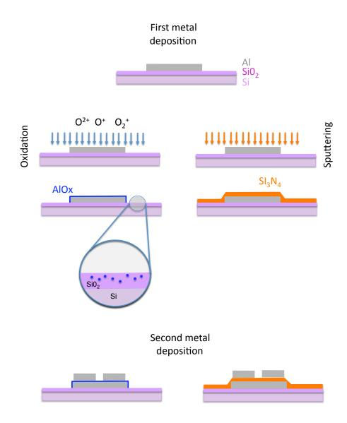
**Fig. D.1.** Fabrication steps of microwave capacitors made of a first floating electrode, either plasma oxidized (left) or covered with sputtered Si<sub>3</sub>N<sub>4</sub> layer (right), and then covered by two overlapping electrodes. Process steps, materials, and chemicals species involved are indicated in the drawings. The circular inset on the left points out an unexpected technical problem encountered during fabrication (see text).
