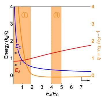
Fig. 2.2. Josephson (red line) and charging (blue line) energies, as well as anharmonicity  $\eta$  (orange line) as a function of  $E_J/E_C$  for  $\nu_{01}(\delta=0,N_g=1/2)=17$  GHz. Orange areas correspond to an anharmonicity larger than 10%, which is the minimum target value for the experiment.
