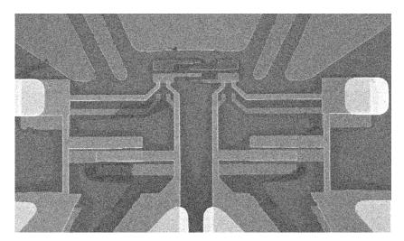
**Fig. 2.17.** Scanning electron micrography of the central part of the quantroswap obtained after double angle evaporation of aluminum through the mask defined in Fig. 2.16.
