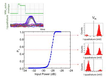
**Fig. 4.14.** Switching probabilities  $P_S$  as a function of the microwave signal power and distribution of the quadrature amplitude of the reflected signal for three different values of  $P_S$  10%, 50%, and 90%. Top right: oscillograms of the microwave pulse envelope (green) and of on of the quadratures of the reflected signal.
