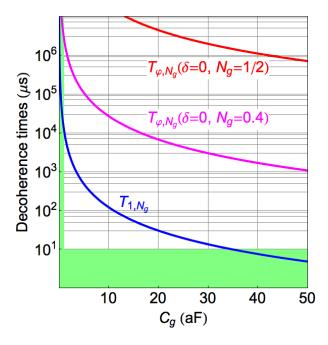
Fig. 2.6. Gate line contribution to decoherence as a function of  $C_g$  for  $E_J = 0.51$  K  $E_C = 0.97$  K:  $T_1$  (blue) is calculated at the optimal point whereas  $T_{\varphi}$  is calculated at  $\delta = 0$  in the relevant range  $N_g \in [0.4, 0.5]$ . The left green area is discarded for power availability reason, while the bottom one corresponds to  $T_1$  shorter than our target value  $10\mu$ s.
