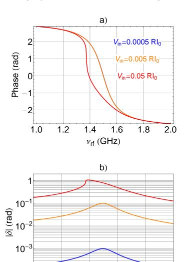
Fig. 5.7. Response of the Blochonium oscillator to microwave excitation as a function of the probe signal frequency for three drive amplitudes  $|2V_{in}/(RI_0)|=0.001$  (blue), 0.01 (orange) and 0.1 (red): phase of the reflected signal (a) and amplitude  $\gamma_a$  of oscillations (b) for  $\nu_p=1.5$  GHz and Q=10.
