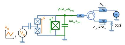
Fig. 5.4. Electrical scheme of the Blochonium circuit. A 50  $\Omega$  source applies an incoming wave of amplitude  $V_{\rm in}$  to a quantronium-like sample. This wave is reflected on the Blochonium oscillator and propagates through a circulator to a 50  $\Omega$  amplifier (50  $\Omega$  resistor on the figure).
