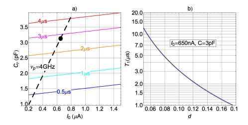
Fig. 2.9. Readout circuit induced relaxation. a) Iso- $T_1$  contours (colored lines) in the  $I_0 - C_r$  plane at optimal point, and assuming a 50 $\Omega$  impedance for the readout line. Dashed line corresponds to the target  $\nu_p = 4$  GHz selected on Fig. 2.8. b)  $T_1$  as a function of d for the selected parameters indicated by a dot in panel a.
