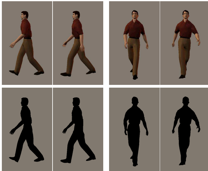
Figure 4.1: Examples of ambiguities in silhouettes: different 3D poses can have very similar image observations, causing the regression from image silhouettes to 3D pose to be inherently multi-valued. The legs and the arms are reversed in the first two images, for example.
