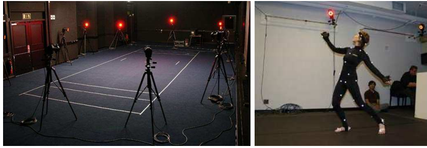
Figure 1.2: A standard multicamera optical motion capture setup. (Left) Several cameras are used to record the position and motion of different joints on the body. (Right) A special costume with reflective markers located at the joint positions is used by an actor who performs the motion.
