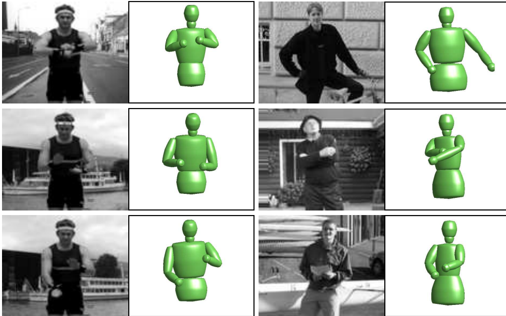
Figure 6.8: Pose reconstructions on real unseen images. The images on the left are taken from a test sequence in our motion capture dataset which includes similar gestures made by another person, while the ones on the right are example images obtained using Google image search.
