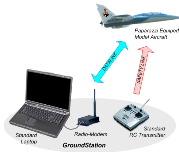
Figure A.1: The basic elements needed for the Paparazzi system to operate.
