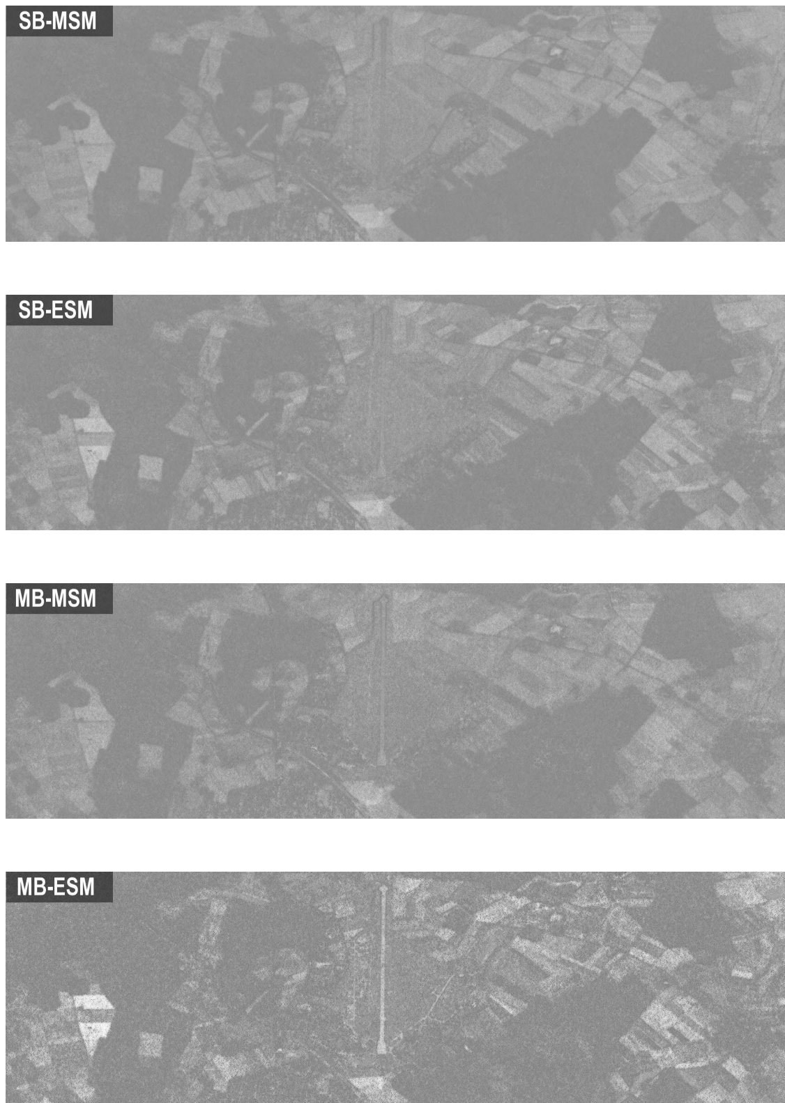
Figure 4.16: Non-filtered data: Local scattering mechanisms correlation \rho_{\omega} images for N = 7^2 . From top to bottom: SB-MSM, SB-ESM, MB-MSM, MB-ESM.
