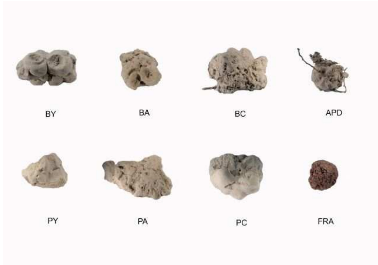
Figure 23 Examples of the different macroaggregate types separated from the 5–12.5 mm size fraction: (BY) young biogenic; (BA) aged biogenic; (BC) colonized biogenic; (APD) associated with plant debris; (PY) young physicogenic; (PA) aged physicogenic; (PC) colonized physicogenic; (FRA) fragile rounded aggregates. All aggregates shown here are from the beech-fir forest, except FRA which is from the pine forest
