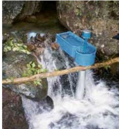
Figure I.4 : Petite turbine hydraulique de 200 W [I.7]
