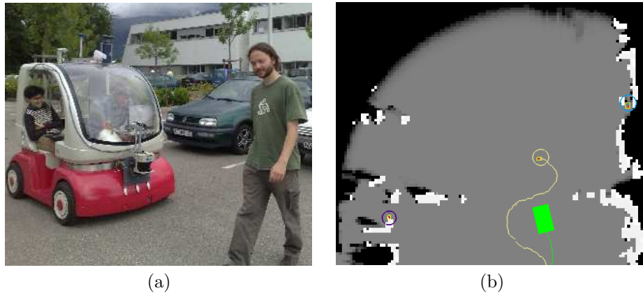
Figure 3.7: (a)The vehicle in the parking lot at INRIA Rhône-Alpes and a moving pedestrian; (b) The extracted occupancy grid, with the vehicle in green and the tracked moving obstacle in yellow.
