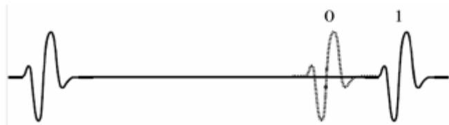
Figure I. 8: Principe de la modulation PPM.
