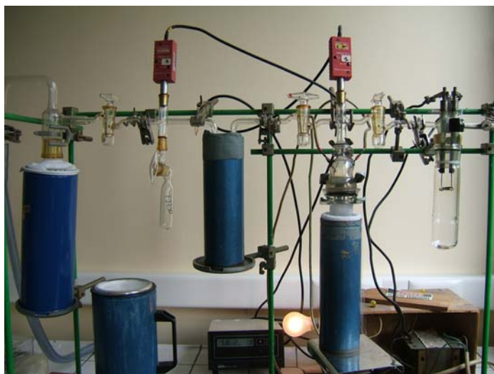
Figure 3.1.1.1 Line for oxygen extraction from the sulphate for \delta^{18}\text{O}_{\text{SO}_4} analyses
