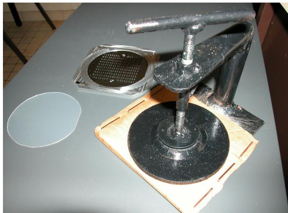
Fig.5.3.3. Press for curing the silicon for obtaining a homogenous film thickness.
