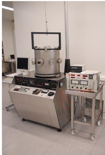
Fig.2.6. Evaporation system (Veeco 770) at LAAS-CNRS.
