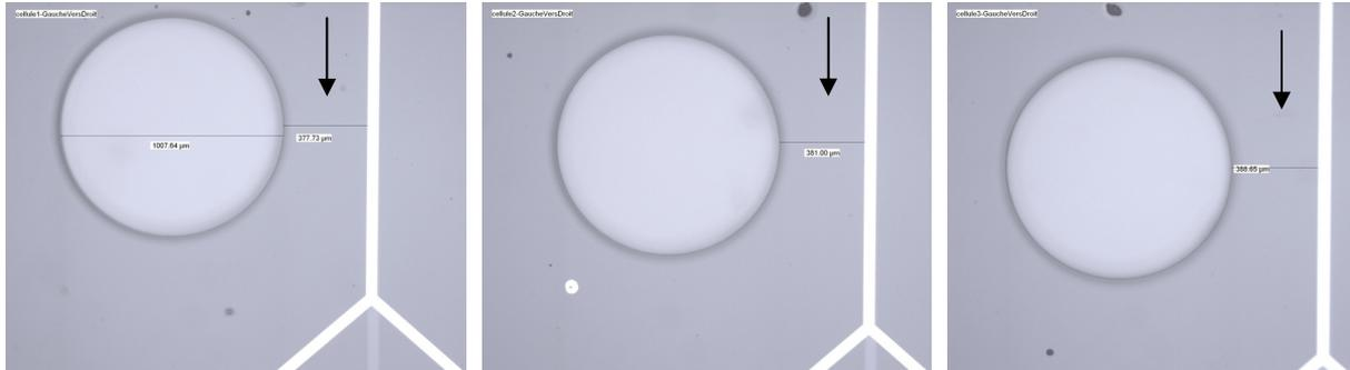
Fig.5.4.4. Alignment of PDMS using modified mould taking into account the shrinkage ratio.
