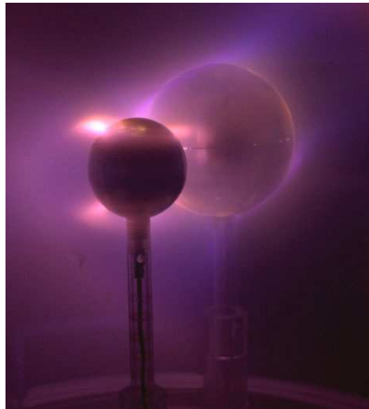
Fig. 4. Interaction between a magnetized star (the large sphere) and a planet (the small one). On the large sphere (the cathode), the electrons are emitted around the magnetic poles which are tilted versus the vertical axis. A “coronal hole” may be seen exactly where the magnetic pole stands. On the small sphere (the anode), a ring current surrounds the “planet” closing on the auroral ovals, similar to the Van Allen belt (credit: G. Gronoff, LPG). Colour version of this figure is available in electronic edition only.
