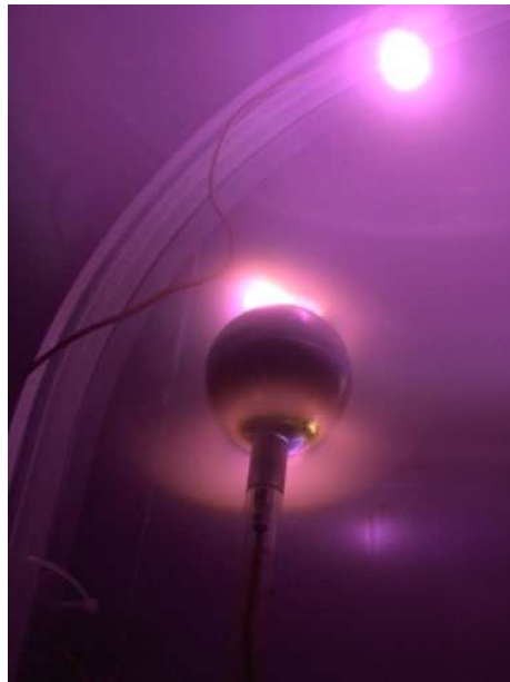
Fig. 5. The cathode (the electric duct at the top of the screen) faces a magnetic pole of the small sphere, representing Uranus. On the “dayside” of this planet-like, an auroral spot develops at the place of the magnetic pole. On the “nightside”, one sees an auroral oval (credit: G. Gronoff, LPG). Colour version of this figure is available in electronic edition only.
