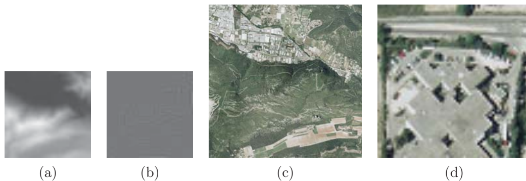
Figure 5.6: Level 1 approximate reconstruction: a) the extracted DEM, b) difference of the extracted with the original DEM, c) the texture, d) the magnified texture.
