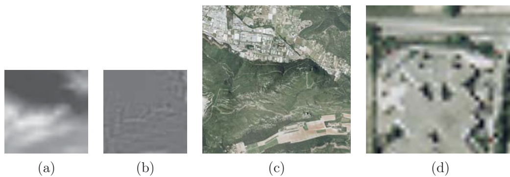
Figure 5.7: Level 2 approximate reconstruction: a) the extracted DEM, b) difference of the extracted with the original DEM, c) the texture, d) the magnified texture.
