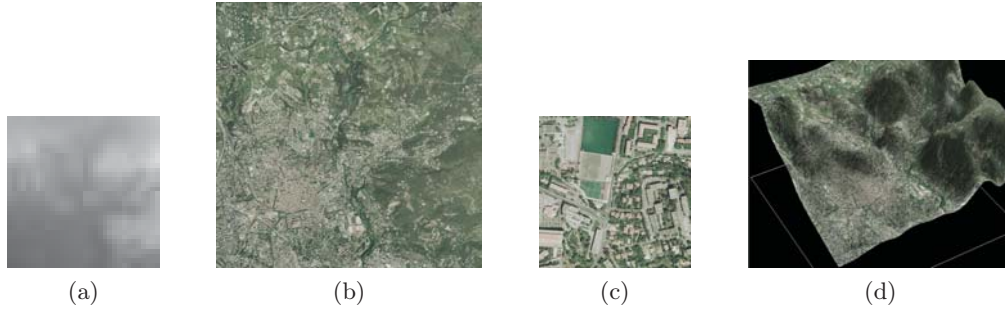
Figure 6.5: Example images: a) 32 \times 32 DEM, b) 3072 \times 3072 pixel texture, c) a 256 \times 256 pixel magnified detail of (b) at (1000, 1500) coordinates, d) a corresponding 3D view.
