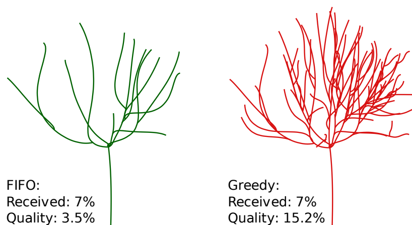
Figure 3.13 – Example showing the structure of the same tree of the scene better packetized by the Greedy strategy.
