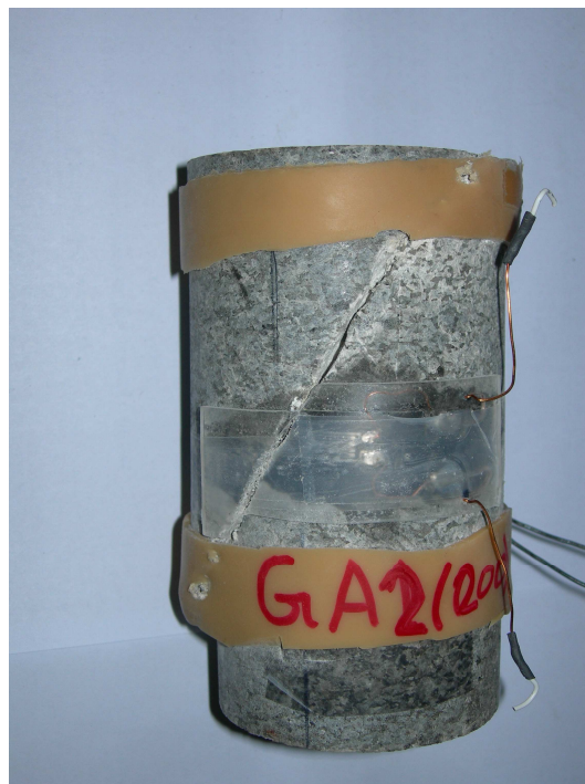
Figure 4.26: Specimen Ga2 (200) after ultra high triaxial test. The sharp, planar failure surface is obvious in this photo.
