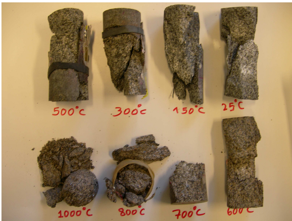
Figure 6.17: A general view of thermally treated specimens after uniaxial testing. Notice the obvious colour change and failure pattern from the intact rock to the specimen thermally treated to 1000°C.
