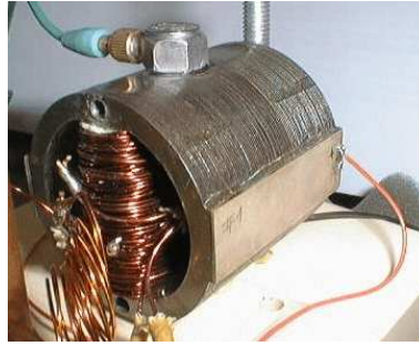
FIGURE 1.22 – Prototype monophasé statique [15]
