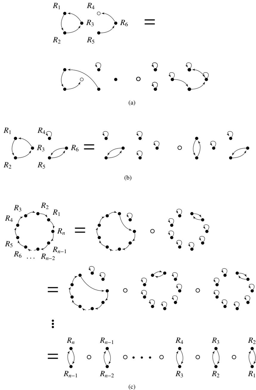
Figure 7.11: Sequentializing reversible parallel copies: (a) after sequentializing the chain  $R_5 \rightarrow R_6 \rightarrow R_4$ ,  $R_5$  is free and used to break the 3-cycle; (b) there are only cycles and no free register: swaps must be used; (c) general case for a  $n$ -cycle when there is no free register.
