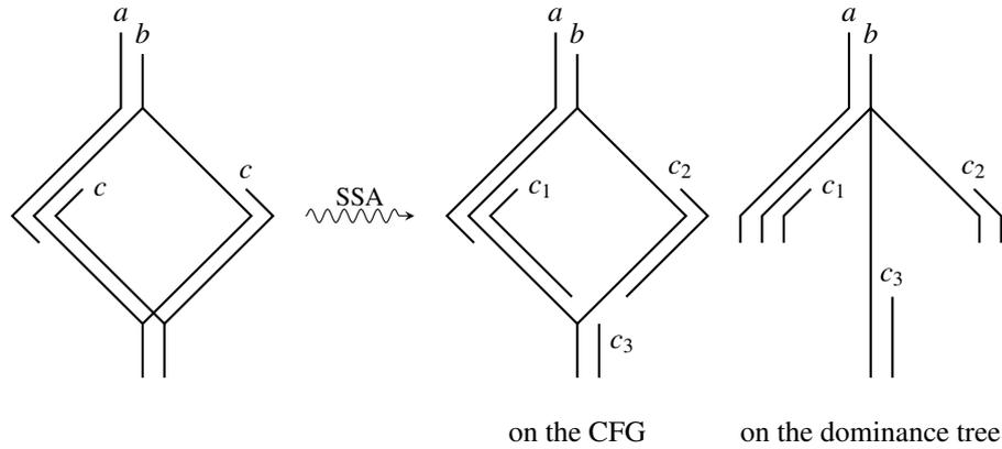
Figure 2.15: Live-ranges of the program of Figure 2.14 and its version under SSA.  $c_1$  and  $c_2$  stop at the end of their definition blocks, while  $c_3$  starts at the beginning of the block with the  $\phi$ -function (see note page 28), hence they are subtrees of the dominance tree.
