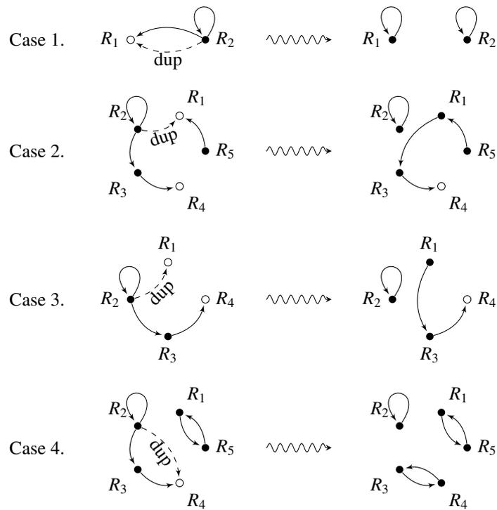
Figure 7.10: The four cases of function `De_compose`. The dashed arrow labeled “dup” shows the choice of *dest* when duplicating *source* register  $R_2$  on the left parallel copies. The graphs on the right show the state of the parallel copy after adding copy “dup” to the predecessor basic block  $B_s$ . Empty bullets show registers not holding live variables at the end of  $B_s$ .
