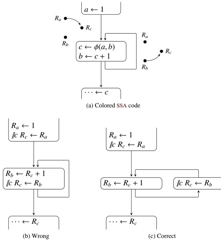
Figure 7.6: Lost copy problem: (a)  $a, b$  and  $c$  reside in different registers; the back-edge of the loop is critical. (b) parallel copies are moved up (at the source of the edges), leading to incorrect value in  $c$  at the exit of the loop (one “+1” too much). (c) a correct way to go out of SSA is to move up the parallel copy at entry point, and to split the critical edge to place the other one.
