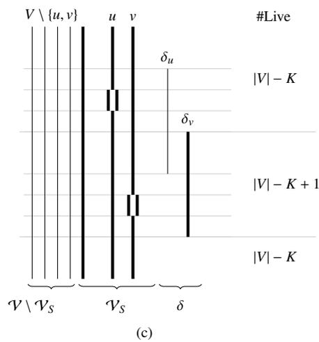
Figure 4.6: Different configurations for the reduction with  $h = 1$ : (a) only  $u$  is spilled, (b) both  $u$  and  $v$  are spilled, (c) none of them are spilled. Non-spilled variables are in bold and  $R = |\mathcal{V}| - K + 1$  registers.
