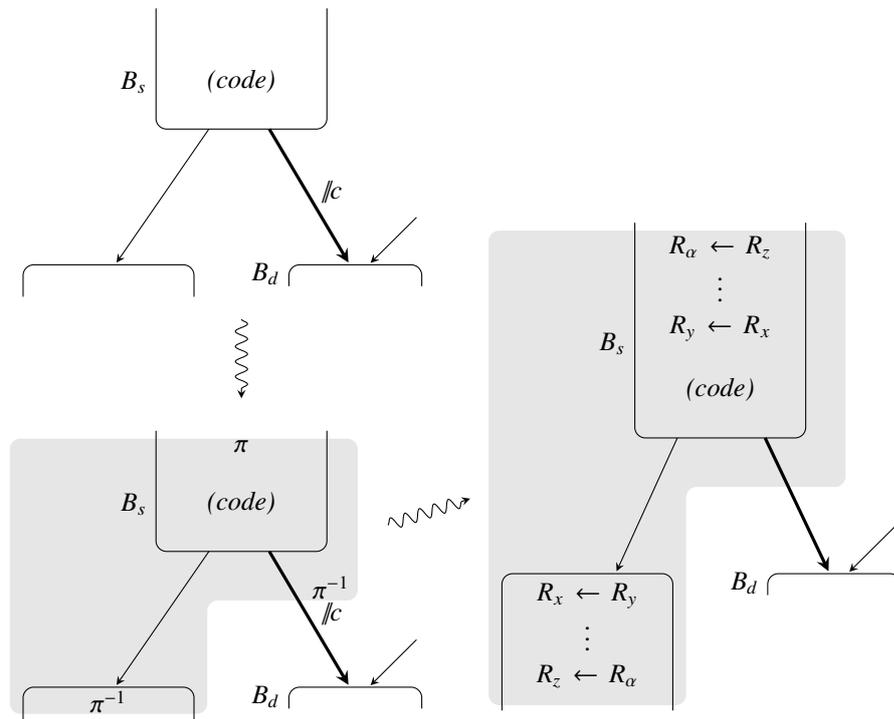
Figure 7.13: Region recoloring: to move up  $//c$ , a region (grayed) is chosen,  $\pi$  is added at the entry, and  $\pi^{-1}$  at the exits. On the critical edge,  $\pi^{-1}$  and  $//c$  cancel each other. The other entry and exit points can be chosen at convenience inside basic blocks.
