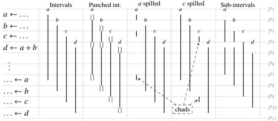
Figure 4.2: Example of punched intervals. When spilled, they leave small intervals (chads) at their definition and uses points. The chads count in the register pressure hence spilling  $a$  is not equivalent as spilling  $c$ : Maxlive stays at 4 with the former, but drops to 3 with the latter.
