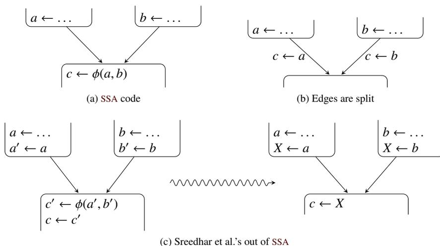
Figure 7.1: Going out of SSA: (a) original SSA code. (b) going out of SSA with the semantics of the  $\phi$ -functions. (c) going out of SSA *à la* Shreedhar.
