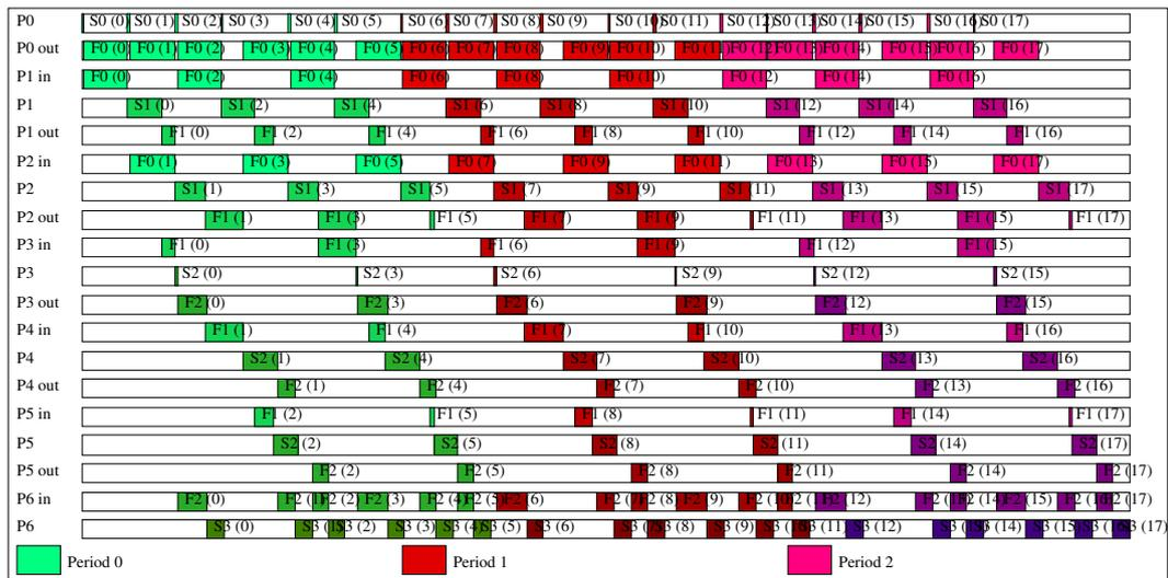
Figure 4.8: Gantt diagram of a schedule without critical resource.
