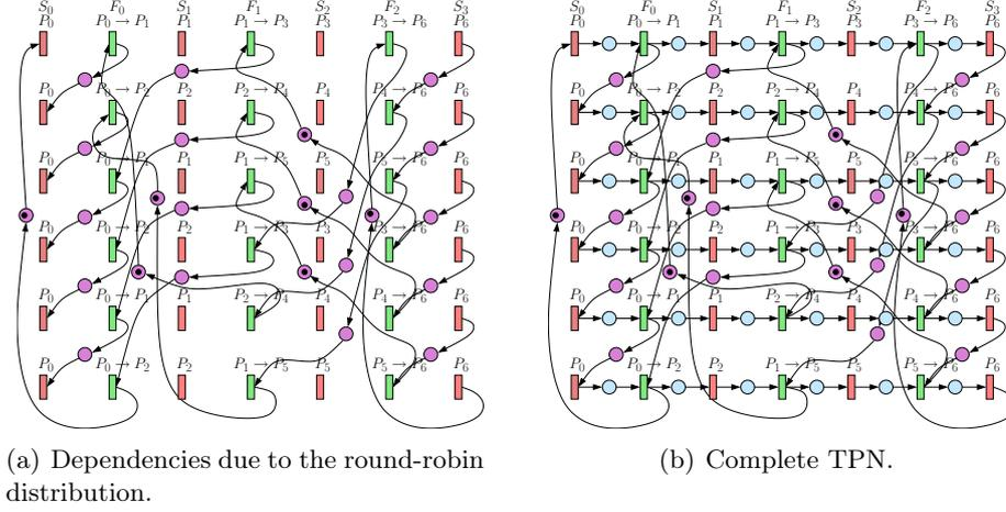
Figure 4.5: TPN of Example A for the model without overlap.
