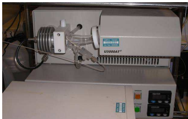
Fig. 3.17 detail of the ultrasonic spray chamber used in this work.
