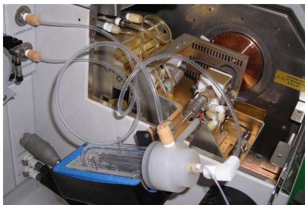
Fig. 3.4 Nebulizer, spray-chamber, torch and sampler cone (upper view).
