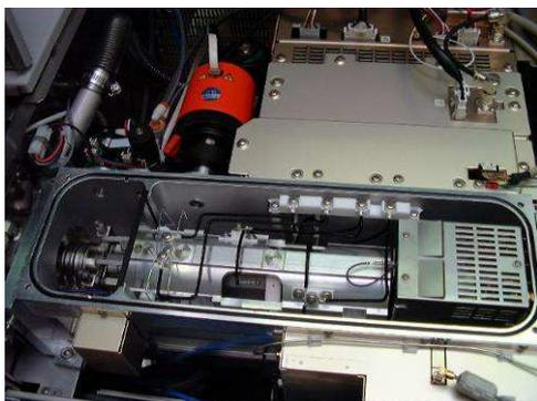
Fig. 3.11 Quadrupole mass analyser system of Agilent 7500.
