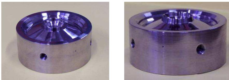
Figure 4.4 The Nickel-270 melting head used in this work.
