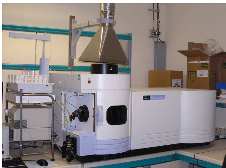
Fig. 3.18 ICP-OES system coupled with an ultrasonic nebulizer used in this work.
