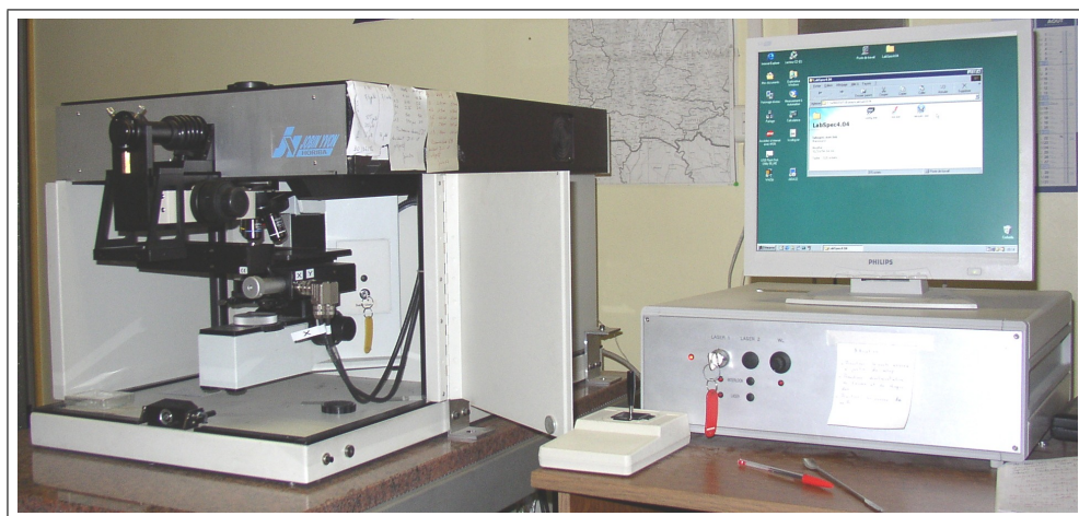
Figure 2.4: The Jobin Yvon Labram Infinity (LI) spectrometer at the LADIR, working in microscopic configuration
