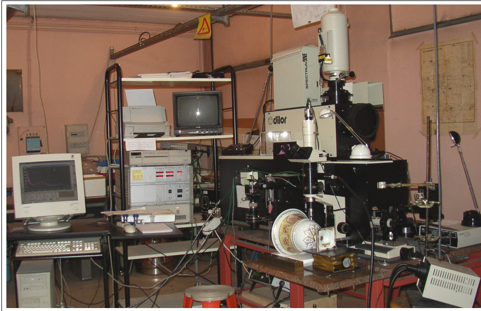
Figure 2.5: The Dilor XY1 spectrometer at the LADIR, suitable for working both in microscopic and macroscopic configuration
